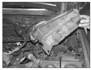
5. Remove the crank case vent from air box then remove the two 8mm bolts that reatin the air box to vehicle. Then remove air box from vehicle as shown.
