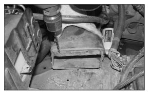
13. Remove the heat shield and drill two 1/4" holes were you marked in the previous step.
