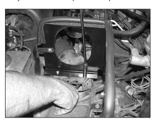
14. Re-install the heat shield onto the vehicle then mount the fresh air duct to the heat shield with the provided hardware as shown.
