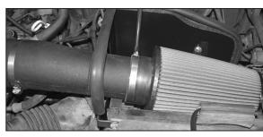
17. Install the air filter onto the new intake tube as shown.
