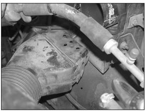
4. Remove the fresh air intake tube from the bottom of air box as shown.
