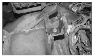
10. Install the provided bracket (07879) onto the air box mounting bracket as shown using one of the the bolts that was removed in step 5.
