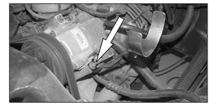
7. On vehicles that come equipped with A/C, remove the front lower A/C mounting bolt. Then secure the saddle bracket assemble from step 6 onto vehicle as shown.
