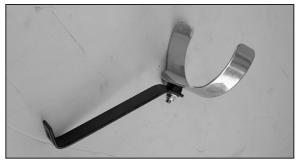
6. On vehicles that come equipped with A/C, assemble the saddle bracket onto bracket (07164) as shown.
