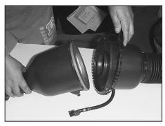
9. Open the air cleaner assembly and isolate the mass air sensor assembly.
