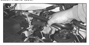
4b. On models with 5.4L engines, detach the idle air control and crank case vent hose from the stock intake tube.
