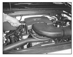
2. Loosen and remove the three bolts that retain the throttle body cover, then remove the cover.
