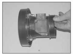
27. Attach the mass air adapter to the mass air sensor using the gasket and provided hardware.
