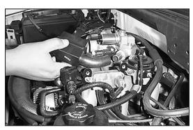
4a. On models with 4.6L engines, detach the air bypass valve and crank case vent hose from the stock intake tube.
