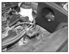
22. Install the saddle bracket assembly onto the protruding stud as shown, secure into place using the provided hardware.
