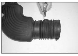
19. Remove the air temp. sensor from the stock air intake tube as shown.
