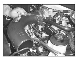
25. On models with 5.4L engines, install the idle air control and crank case vent hose onto the appropriate fittings on the K&N® intake tube, secure with the hose clamps provided.
