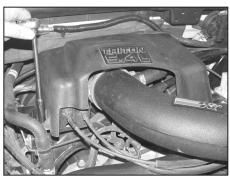
33. Reinstall the engine cover removed in step #2.
