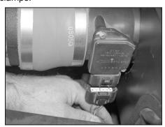
30. Reconnect the primary and secondary mass air electrical connections.
