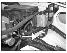
15. Remove the 6mm bolt that retains the cruise control onto the vehicle.
