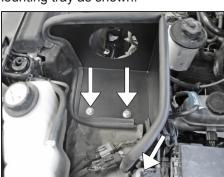
18. On vehicles equipped with cruise control, set the heat shield into position on the air filter mounting bracket. Then secure the heat shield with the provided hardware as shown.
