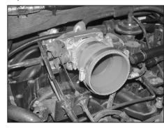
23. Using the provided hose clamp, attach the silicone hose (08724) to the throttle body.
