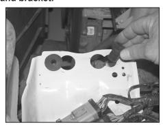
17. Install the two nut inserts into the air box mounting tray as shown.
