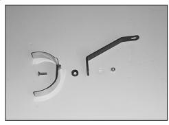
21. Assemble the saddle to the appropriate bracket using the provided hardware as shown.
