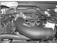
24. Install the K&N<sup>®</sup> intake tube onto the throttle body and tighten the hose clamp.
