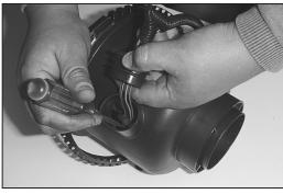
10. Slide the rubber grommet back and disconnect the primary mass air sensor electrical connection, using a flat blade screwdriver.
