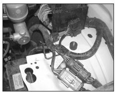
15a. On vehicles without cruise control, install the rubber mounted stud onto the vehicle as shown.
