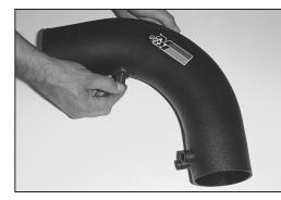
20. Using the provided grommet, install the air temperature sensor into the K&N<sup>®</sup> intake tube.
