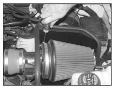
32. Install the K&N<sup>®</sup> air filter onto the mass air adapter and secure it with the provided hose clamp.
