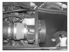
29. Attach the mass air assembly to the intake tube. Secure the mass air assembly and saddle bracket to the intake tube using the provided hose clamps.
