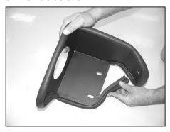
14. Install edge trim onto the heat shield as shown. Trim if needed.
