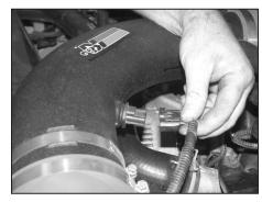
31. Reconnect the air temp. sensor electrical connection.
