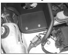
18a. On vehicles not equipped with cruise control, set the heat shield into position on the air filter mounting bracket and then secure the heat shield with the provided hardware as shown.
