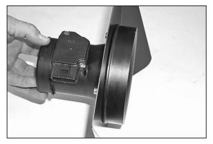
8. Assemble the mass air adapter, gaskets, heat shield and mass air sensor as shown.
