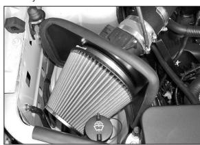
21. Install the heat shield assembly onto the K&N® intake tube and tighten the hose clamp as shown. NOTE: Adjust heat shield for best clearance before tightening.
