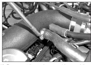
19. Re-connect the crankcase vent hose and the idle bypass hose then secure with the provided hose clamp to the K&N® intake tube as shown.
