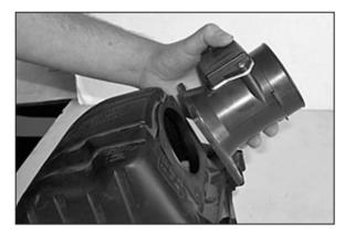
7. Loosen and remove the four bolts that secure the mass air sensor, then remove the mass air sensor as shown.
