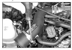
17. Secure the intake tube to the saddle bracket assembly with the provided hose clamp.
