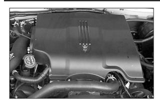
23. Re-install the engine cover then secure with the two 11mm nuts that were removed in step 3.
