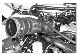
5. Loosen the hose clamp at the throttle body and at the mass air sensor, then remove the stock air intake tube as shown.
