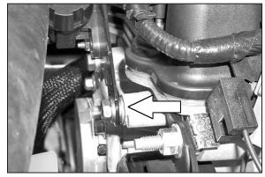
14. Install the new bracket between the cylinder head and purge solenoid bracket then install the two provided washers behind the purge solenoid bracket (see arrow), then secure with the two factory bolts.
