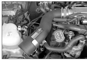
16. Install the K&N® intake tube onto the throttle body then line it up with the saddle bracket assembly as shown.
