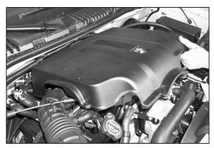
3. Loosen and remove the two 11mm nuts that secure the engine cover, then remove the cover as
