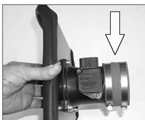
10. Assemble the silicone hose (08630) and the hose clamps onto the heat shield assembly as shown.
