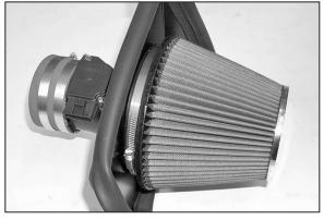
20. Install the  $K\&N^{\otimes}$  air filter onto the heat shield assembly as shown.
