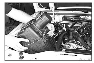
6. Using a screwdriver, pry up the bottom of the air cleaner to release the air cleaner from the stock grommets, then remove the air cleaner assembly as shown.
