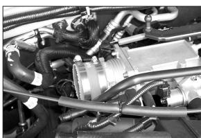
11. Install the silicone hose (08434) and the hose clamps onto the throttle body as shown.
