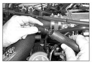
18. Remove the factory hose mender from vent hose as shown.
