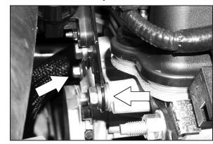
13. Remove the two bolts with a 13mm wrench that secure the purge solenoid to the front of the cylinder head as shown.
