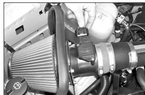
22. Re-connect the mass air sensor electrical connection as shown.
