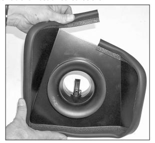
9. Apply the trim seal to the heat shield assembly as shown. Trim if needed.
