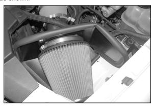
33. Install the K&N® Filtercharger onto the mass air
