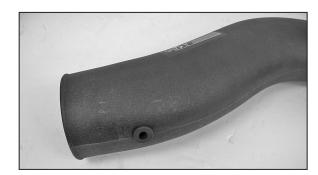
18. Install the provided grommet into the new intake tube as shown.
