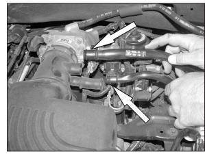
4. Remove the idle air control and the crankcase vent hose from the stock intake tube.
