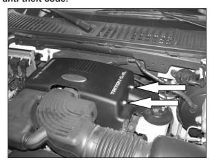
2. Loosen and remove the two bolts that retain the engine cover, then remove the cover.
