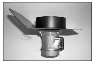
27. Assemble the heat shield and filter adapter onto the mass air sensor with the provided hardware.
