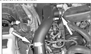
17. Install the new K&N intake tube onto the vehicle and then tighten the provided hose clamps at the throttle body and saddle bracket.
