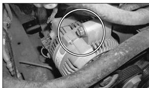
14. Remove the bolt that retains the alternator onto the motor.
