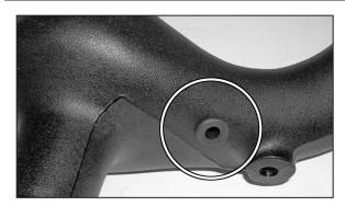
10. Install the provided grommet into the new K&N intake tube as shown.
