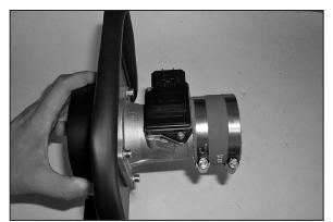
29. Install the silicone hose onto the mass air sensor with the provided hose clamps
