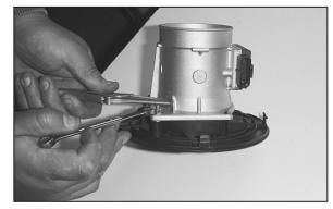
26. Using a pair of small vise grips or pliers, hold the stud while using a 10mm wrench to loosen the nuts, then remove the mass air sensor from the retaining plate.
