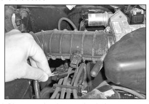
2. Disconnect the air temp. electrical sensor as shown.
