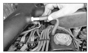
22. Connect the new silicone hose onto the valve cover and intake tube as shown.
