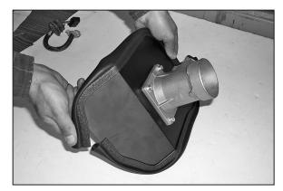
28. Install the edge trim onto the heat shield as shown. Trim if needed.
