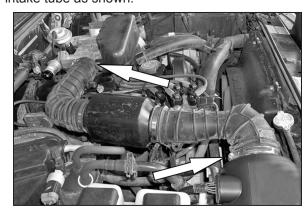
6. Loosen the two hose clamps at the throttle body and air box.
