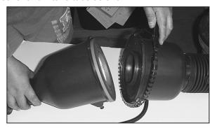
23. Open the air cleaner assembly and isolate the mass air sensor assembly.
