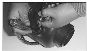
24. Slide the rubber grommet back and disconnect the primary mass air sensor electrical connection, using a flat blade screwdriver.
