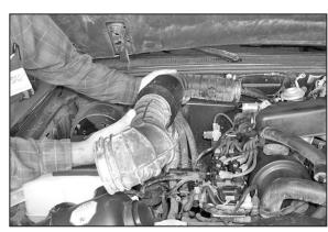
7. Remove the intake tube as shown.
