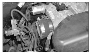
12. Install the provided silicone hose onto the throttle body with the provided hose clamps.
