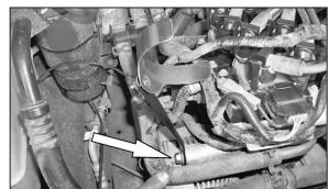
15. Install the saddle bracket assembly onto the alternator with the bolt that was removed in the previous step.
