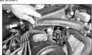
21. Remove the crank case vent hose from the valve cover as shown.
