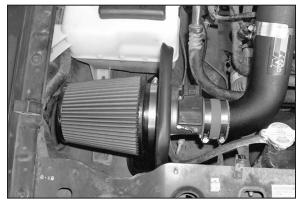
31. Install the K&N Filtercharger onto the mass air assembly as shown.
