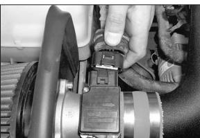
33. Reconnect the mass air electrical sensor as shown.
