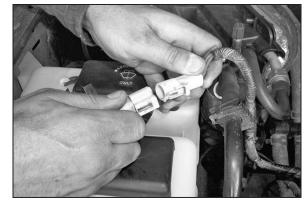
32. Connect the mass air pigtail to the main wire loom as shown.
