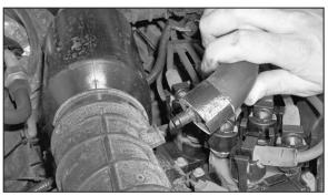
3. Remove the crank case vent from the intake tube as shown.
