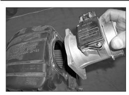
11. Loosen and remove the four hex bolts that secure the mass air sensor, then remove the mass air sensor from the air cleaner as shown.
