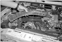
6. Loosen the hose clamps at the throttle body and at the mass air sensor, then, remove the stock rubber intake tube as shown.
