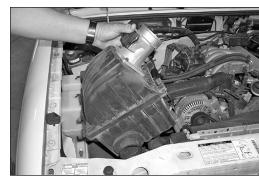
7. Slide a flat blade screwdriver in between the air cleaner and the air cleaner mounting tray. Pry downwards on the tray, while pulling upwards on the air cleaner assembly to release the assembly from the retaining grommets in the tray.
