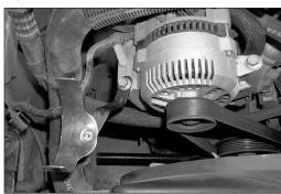
16. Using the bolt removed in step 9, secure the saddle bracket assembly to the alternator as shown. Do not tighten completely at this time.
