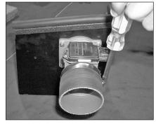
17. Install the silicone hose and the #44 hose clamp onto the mass air sensor as shown.
