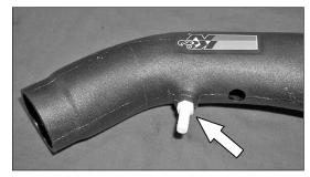
18. Install the 3/8" vent into the threaded boss on the K&N® intake tube as shown.
