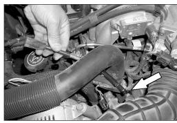
4. Disconnect and remove the crank case vent hose from the stock rubber intake tube as shown.
