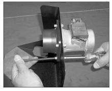
12. Assemble the mass air adapter, heat shield, gaskets and the stock mass air sensor using the provided hex bolts and wave washers as shown.
