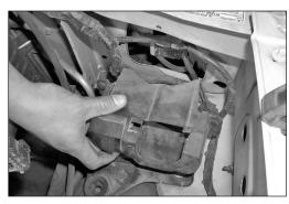
8. Pull firmly on the air inlet duct to release the duct from the radiator core support as shown.
