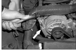
9. Loosen and remove the lower front alternator hex bolt as shown.
