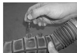
10. Remove the air temperature sensor from the stock rubber intake tube as shown.
