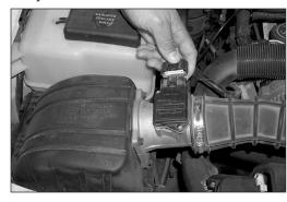
2. Disconnect the mass air sensor electrical connection as shown.
