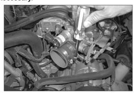
14. Install the silicone hose and hose clamps onto the throttle body as shown.
