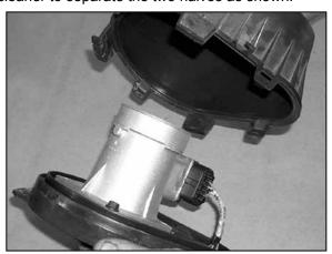
9. Using a flat blade screwdriver, depress the tabs to release the mass air sensor cover from the mass air sensor base plate as shown.
