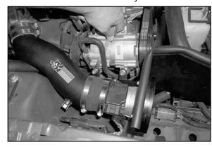
24. Line up the support bracket with the A/C compressor and secure with the original bolts removed in step 13 using a 13mm wrench.
