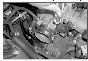
22. Install the provided silicone hose and hose clamps onto the throttle body as shown.
