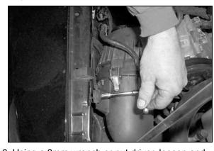
6. Using a 8mm wrench or nut driver, loosen and remove the bolt that secures the air cleaner to the inner fender as shown.
