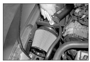
26. Install the K&N® Air filter and secure with the provided hose clamp as shown. Adjust intake tube and tighten all clamps completely.
