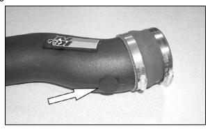
19. On 2001 vehicles install the rubber plug into the hole on the K&N® intake tube.
