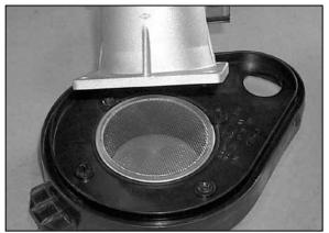
12. Using a 10mm wrench or nut driver loosen and remove the two bolts that secure the mass air sensor, then, remove the mass air sensor from the base plate as shown.
