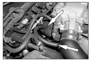
25. Install the provided hose onto the vent on the cam cover, then, reconnect the hose to the 3/8" vent on the K&N® intake tube.
