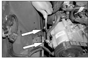
13. Using a 13mm wrench loosen and remove the two lower A/C compressor bolts as shown.
