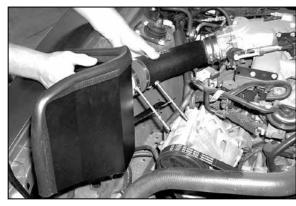
23. Slide the K&N® intake assembly into the silicone hose on the throttle body as shown.
