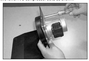
14. Using the provided hardware assemble the mass air adapter, heat shield, gaskets, and the mass air sensor as shown using a 10mm wrench or nut driver.
