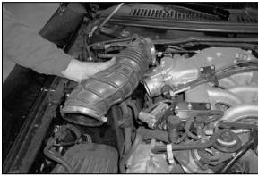
5. Using a flat blade screwdriver loosen the hose clamps at the throttle body and at the air cleaner, then, remove the rubber intake hose as shown.
