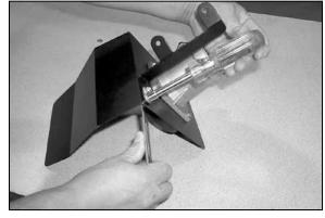
15. Using the provided hardware, assemble the support bracket onto the heat shield using a 10mm wrench as shown.
