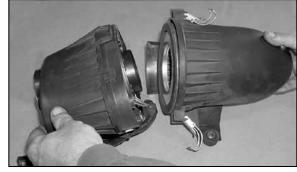
8. Release the over-center clamps on the air cleaner to separate the two halves as shown.
