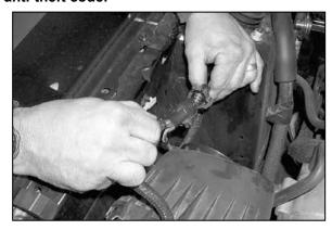
2. Disconnect the secondary mass air sensor electrical connection as shown.
