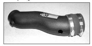
17. Install the provided silicone hose and hose clamps onto the K&N® intake tube as shown.
