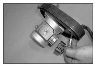
10. Disconnect the mass air sensor electrical connection from the mass air sensor as shown.
