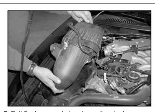
7. Pull firmly upwards to release the air cleaner from the factory grommets, then remove the air cleaner as shown.
