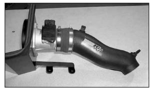
21. Slide the K&N® intake tube onto the mass air sensor as shown, but do not tighten completely.
