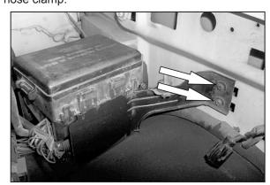
15. Loosen and remove the two bolts that secure the fuse box bracket to the inner fender as shown. (see arrows)
