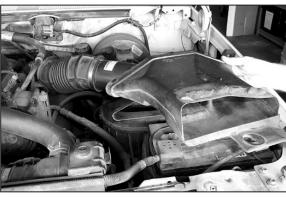
2. Loosen and remove the bolt on the radiator core support, then remove the air inlet duct as shown.
