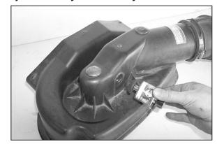
24. Remove the stock filter minder and the stock grommet from the stock air cleaner top as shown.
