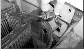
5. To remove the air temperature sensor, turn the sensor ½ turn, then, pull the sensor out of the lower air cleaner assembly as shown.
