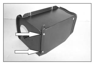
10. Using the provided hardware, install the straight bracket onto the bottom of the K&N $^{\odot}$  heat shield as shown.
