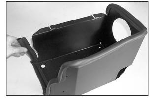
9. Apply the provided trim seal to the  $K\&N^{\otimes}$  heat shield as shown.
