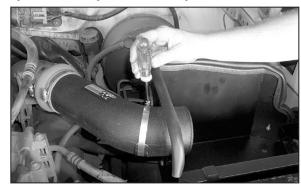
23. Secure the K&N® intake tube to the saddle bracket with the provided hose clamp as shown. NOTE: Do not tighten completely as some adjustment may be necessary.
