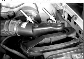
3. Loosen the screws that secure the air cleaner top as shown. (see arrows)
