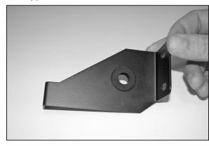
17a. Vehicles that come with twist in air temp sensor, install grommet (08167) into air filter support bracket as shown.
