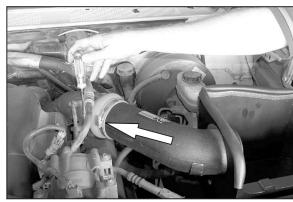
22. Install the K&N® intake tube onto the turbo inlet tube and secure the hump hose with the provided hose clamp.
