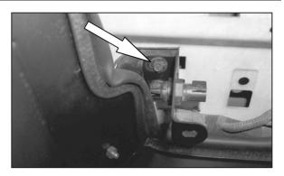
20. Install the air filter support bracket onto the fuse box support bracket using the bolts removed in step 15.
