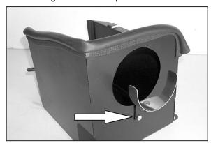
13. Install the saddle bracket assembly onto the  $K\&N^{\circledcirc}$  heat shield using the provided hardware as shown.
