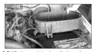
7. Pull firmly upwards to release the lower air cleaner assembly from the retaining grommets, then remove as shown.
