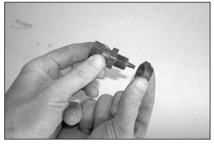
16. Remove the stock retaining nut on the air temperature sensor as shown.
