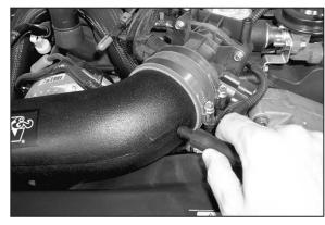
18. On vehicles that come equipped with a second vent line, line up the vent hose on the intake tube and make a mark on the intake tube for drilling.
