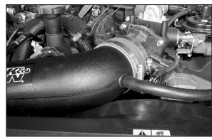
21. Vehicles that come equipped with a second vent line, reconnect as shown
