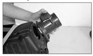
8. Loosen and remove the four bolts that secure the mass air sensor, then remove the mass air sensor as shown.
