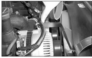
15. Push the wire harness push clip into the hole on the saddle bracket as shown.
