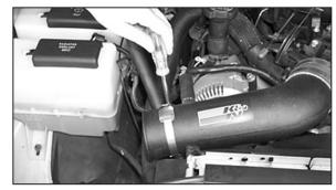
19. Re-install the K&N® intake tube onto the throttle body then secure the intake tube to the saddle bracket assembly with the provided hose clamp.
