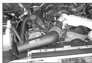
17. Install the K&N® intake tube onto the throttle body and line it up with the saddle bracket assembly as shown.
