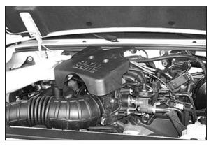
3. Loosen and remove the three bolts that secure the throttle body cover, then remove the cover as shown.
