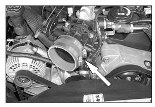
12. Install the silicone hose (08630) and the hose clamps onto the throttle body as shown.
