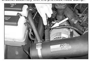
20. Re-connect the crankcase vent hose to the  $K\&N^{\mbox{\tiny 8}}$  intake tube as shown.
