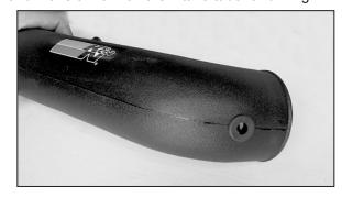
18a. After marking the intake tube, remove the tube from the vehicle and drill a 5/8" hole into the intake tube then install the provided grommet as shown.
