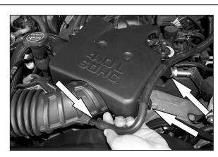
5. On vehicles that come with a second vent line, remove hose from intake tube then release the two clips that retain the hose to the engine cover.
