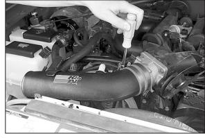
19. Install the  $K\&N^{\otimes}$  intake tube onto the throttle body as shown.
