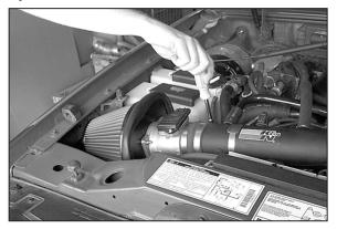
24. Install the heat shield assembly onto the K&N intake tube and tighten the hose clamp as shown
