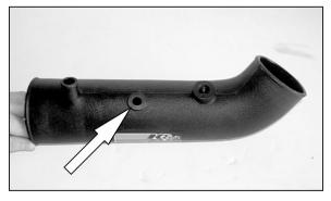
16. On vehicles equipped with an air temp sensor, install the provided grommet into the hole from step 15.
