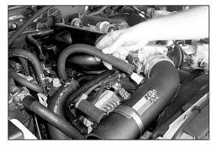
21. Remove the factory CCV hose from the valve cover and install the provided silicone hose onto the valve cover then secure the other end to the K&N® intake tube as shown.
