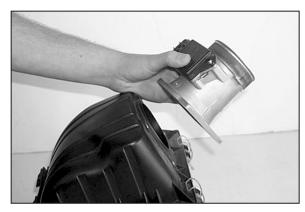
7. Loosen and remove the 4 bolts that secure the mass air sensor then remove the mass air sensor as shown.
