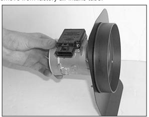
9. Using the provided hardware, assemble the mass air adapter, gasket, heat shield and the mass air sensor as shown.
