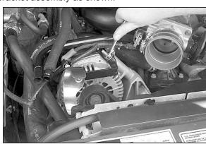
14. Remove the factory alternator stud and install the saddle bracket assembly using the factory stud as show.
