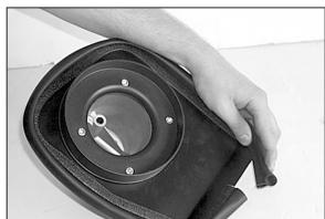
10. Install the trim seal onto the heat shield assembly as shown.
