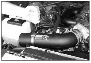
20. Secure the K&N® intake tube to the saddle bracket assembly with the provided hose clamp as shown.
