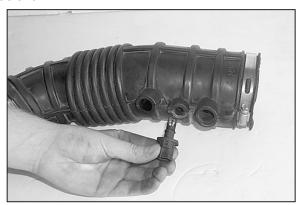
8. On vehicles equipped with an air temp sensor, remove from factory air intake tube.
