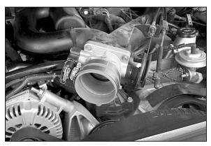
12. Install the silicone hose and hose clamps onto the throttle body as shown.
