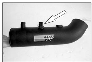
17. Install the air temp sensor into the grommet as shown.
