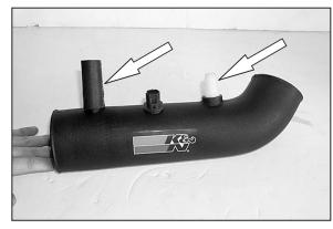
18. Install the rubber hose and 5/8" barbed vent onto the  $K\&N^{\otimes}$  intake tube as shown.
