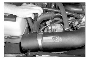
22. Reconnect the air temp sensor electrical connection and the IAC vent hose as shown.
