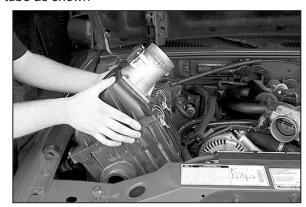
6. Using a screw driver, pry the air cleaner assembly upwards to release the air cleaner from the factory grommets, then remove the air cleaner assembly.
