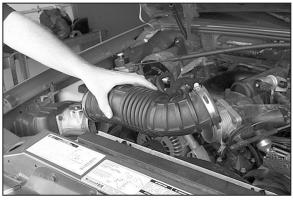
5. Loosen the hose clamps at the throttle body and the mass air sensor, then remove the air intake tube as shown
