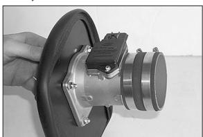
11. Install the silicone hose and hose clamps onto the heat shield assembly as shown.
