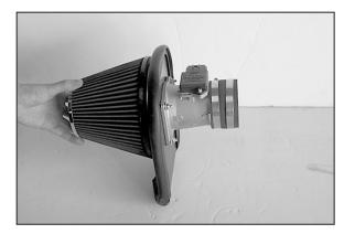
23. Install the K&N Filtercharger onto the heat shield assembly as shown.
