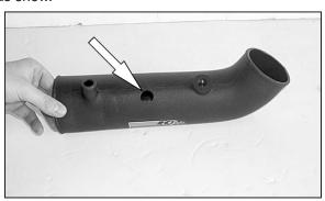
15. On vehicles equipped with an air temp sensor, drill an 11/16" hole on the drill point located on the tube.
