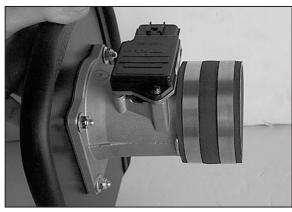
12. Install the silicone hose and hose clamps onto the heat shield assembly as shown.
