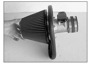
22. Install the K&N<sup>®</sup> Filter onto the heat shield assembly as shown.
