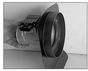
10. Using the provided hardware, assemble the mass air adapter, gaskets, heat shield and mass air sensor as shown.
