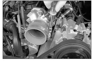
13. Install the silicone hose and hose clamps onto the throttle body as shown.
