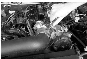
20. Install the K&N<sup>®</sup> intake tube onto the throttle body and secure as shown.
