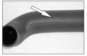
16. On models equipped with an external air temp sensor, drill out the drill point in the  $K\&N^{\otimes}$  intake tube using a 11/16" drill bit.
