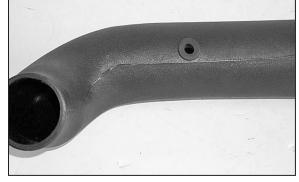
17. Install the provided grommet onto the K&N intake tube as shown.
