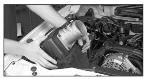
7. Using a screwdriver, pry up on the bottom of the air cleaner assembly to release the air cleaner from the factory grommets, then remove the air cleaner assembly as shown.
