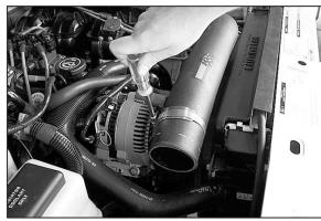
21. Using the provided hose clamp, secure the K&N intake tube to the saddle bracket assembly as shown.
