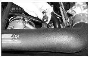
25. Reconnect the air temp sensor electrical connectionas shown.
