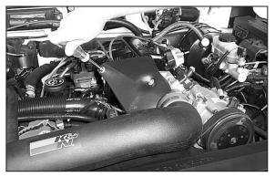
27. Re-install the throttle linkage cover as shown.
