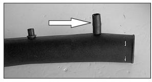
19. Install the rubber hose onto the vent on the  $K\&N^{\circledast}$  intake tube as shown.
