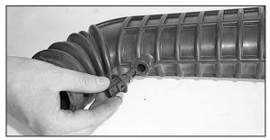
9. Remove the air temp. sensor from the factory intake tube as shown.
