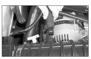
4. Remove the crankcase vent hose as shown.
