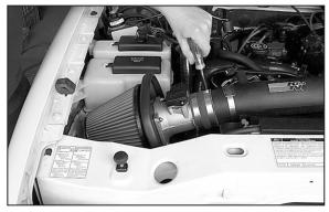
23. Install the heat shield assembly onto the K&N<sup>®</sup> intake tube and tighten the hose clamp as shown.
