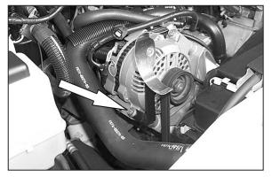
15. Remove the front lower alternator bolt, then secure the saddle bracket assembly using the same bolt as shown.
