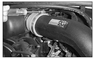
28. Position the intake tube for best alignment and tighten the hose clamp on the stepped hose at the intake tube
