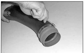
25. Install the hump hose onto the intake tube and tighten hose clamp.
