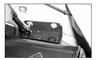
30. Tighten the two bolts that retains the evaporative canister mounting bracket to the inner fender.
