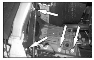
9a. On 2004 and later vehicles loosen and remove the four bolts, which retain the air box-evap canister bracket shown.
