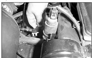
3. Detach the mass air sensor wiring harness from the inner fender apron.
