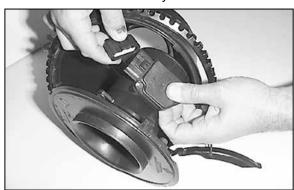
17. Disconnect the primary mass air sensor electrical connection.
