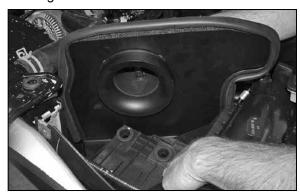
26a. On 2004 and later vehicles, lift up the air boxevap bracket and install the heat shield as shown.
