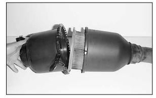
14. Disassemble the air cleaner assembly.
