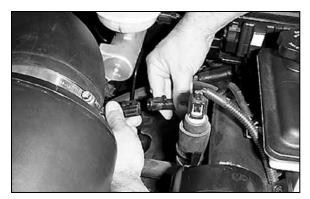
4. Disconnect the secondary mass air sensor electrical connection.
