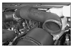
7. Remove the stock intake tube.
