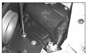
29. Position the heat shield for best alignment and tighten the hardware that retains it.
