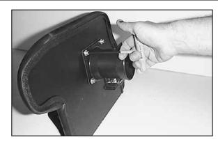
20. Assemble mass air sensor, heat shield and adapter using the gaskets and hardware provided.
