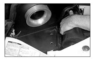
26. Lift up on the evaporative canister mounting bracket and install the heat shield.
