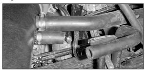
36. Attach the vent hose provided to the small vent fitting on the intake tube.
