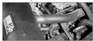
35. Attach the idle air control line to the large vent fitting on the intake tube
