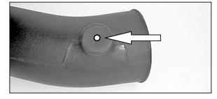
23. On models equipped with an external air temperature sensor, drill out the drill point in the K&N<sup>®</sup> intake tube using a 11/16" drill bit.
