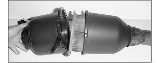
15. Disassemble the air cleaner assembly.
