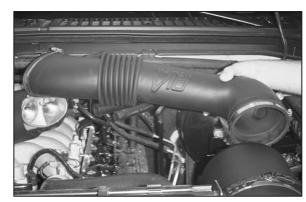
7. Remove the stock intake tube.
