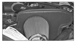
41. Install the Air Filter and tighten the hose clamp. NOTE: Drycharger<sup>®</sup> air filter wrap; part # RF-1020DK is available to purchase separately. To learn more about Drycharger<sup>®</sup> filter wraps or look up color availability please visit http://www.knfilters.com<sup>®</sup>.
