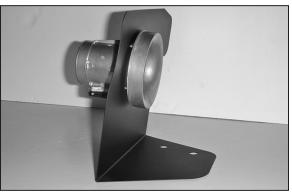
20. Assemble the mass air sensor, heat shield and adapter using the gaskets and hardware provided.
