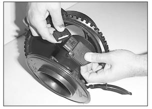
18. Disconnect the primary mass air sensor electrical connection.
