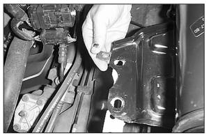
14. Remove the two clip nuts from the evaporative canister bracket lower mounting point. **Note: The clip nuts will not be reused.**
