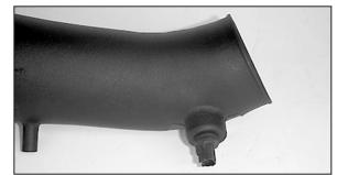
25. On models equipped with an external air temperature sensor, insert the air temperature sensor into the grommet.
