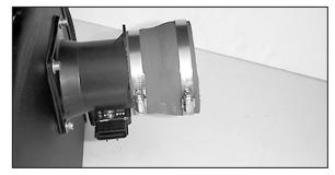
27. Install the stepped hose onto the flange of the mass air sensor and tighten hose clamp.
