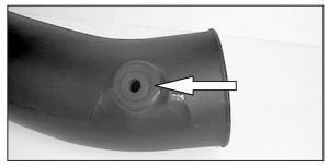
24. On models equipped with an external air temperature sensor, insert the grommet into the hole drilled in the  $K\&N^{\otimes}$  intake tube.
