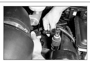
4. Disconnect the secondary mass air sensor electrical connection.
