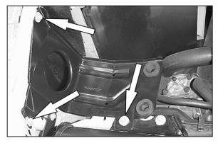
10. Loosen and remove the three bolts that retain the air cleaner mounting bracket.
