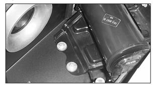
29. Install the provided hardware to retain the heat shield.
