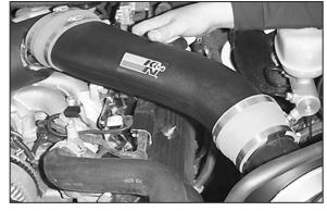
30. Install the intake tube.
