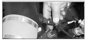
40. On models equipped with an external air temperature sensor, reconnect the air temperature sensor electrical connection.
