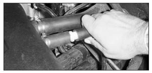
37. Connect the PCV line to the vent hose using the hose mender provided.
