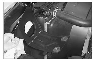
11. Remove the air cleaner mounting bracket. NOTE: On 2004 and later vehicles, this bracket is not removed as it is one piece.
