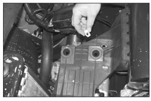
14a. On 2004 and later vehicles remove the clip nuts from under the air box-evap bracket as shown.
