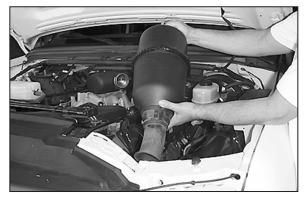
9. Pull upward firmly and remove the air cleaner. NOTE: K&N Engineering, Inc., recommends that customers do not discard factory air intake.
