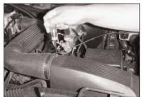
2. Loosen the hose clamp at the air cleaner assembly as shown.
