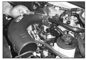
20a. On models with 5.4L engines, install the idle air control and crankcase vent hose onto the appropriate fittings on the intake tube, secure with the hose clamps provided.
