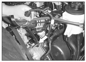
17. Install the saddle bracket assembly onto the protruding stud as shown, secure into place using the hardware provided.
