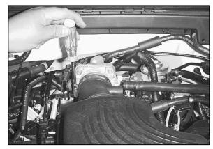
2. Loosen and remove the three bolts that retain the throttle body cover, then remove the cover.
