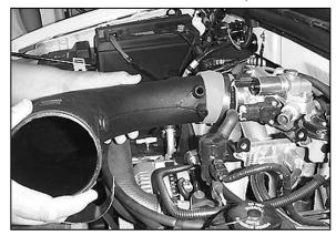
19. Install the intake tube into the small silicone hose and tighten clamp.
