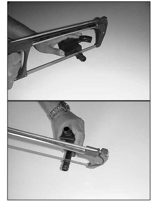
21. On models with 4.6L engines, in some isolated instances where a whistling noise may exist. Cut the flange of the air bypass valve just past the last barb as shown. Reinstall the air bypass valve, attaching it to the appropriate fitting on the intake tube using the 3/4" id hose and hose clamps provided.
