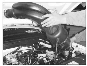
8. Remove the entire stock air intake assembly from the vehicle. **NOTE: K&N Engineering, Inc., recommends that**
