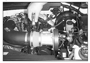
23. Attach the mass air assembly to the intake tube. Secure the mass air assembly and saddle bracket to the intake tube using the hose clamps provided.
