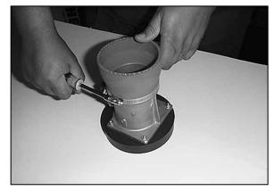
22. Install the large silicone hose onto the mass air sensor and secure with hose clamp provided. NOTE: It may be helpful to apply a slight amount of soapy water solution onto the inner edge of the silicone hose.
