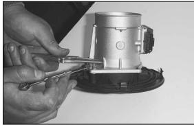
12. Using a pair of small vise grips or pliers, hold the stud while using a 10mm wrench to loosen the nuts, then remove the mass air sensor from the retaining plate.
