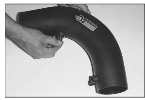
15. Using the grommet provided, install the air temperature sensor into the intake tube.
