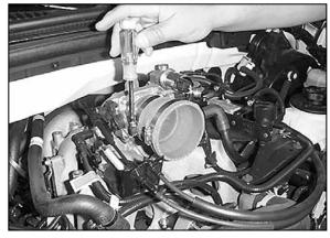
18. Using the hose clamp provided, attach the small silicone hose to the throttle body.
