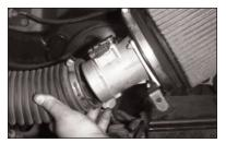
19. Attach the intake tube to the mass air sensor and tighten the hose clamp. NOTE: For best clearance it may be necessary to bend the original airbox mounting bracket away from the air filter.
