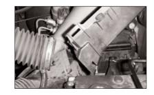
7. Loosen and remove the four nuts that secure the mass air sensor to the airbox top. Remove the mass air sensor from the airbox top.
