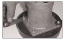
10. Apply the temperature sensor gasket onto the air temperature sensor bracket.
