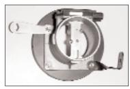
9. Assemble the mass air sensor, mass air adapter. twist bracket and air temperature sensor bracket as shown in the above illustration.
