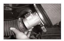
13. Attach the intake tube to the mass air sensor
