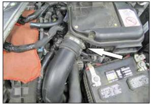
6. Loosen the hose clamp which secures the intake tube to the air box and then disconnect the intake hose from the air box.
