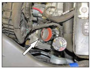
16. Install the provided silicone hose (08108) onto the throttle body and secure with the provided hose clamp. 21. Remove the inlet air temperature sensor from the factory intake tube.
