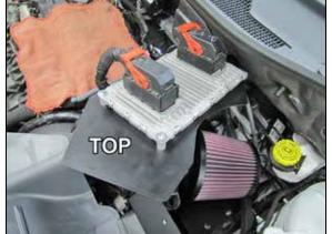
27. Secure the ECU and mounting bracket (083171) and ground strap to the air box lid using the provided hardware as shown.
