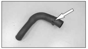
20. Install the provided grommet into the  $K\&N^{\otimes}$  intake tube as shown.
