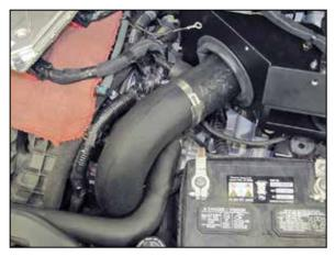
23. Install the K&N<sup>®</sup> intake tube into the silicone hose at the throttle body and then secure the intake tube with the provided hose clamps.
