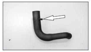
22. Install the inlet air temperature sensor into the grommet installed into the K&N<sup>®</sup> intake tube. NOTE: The inlet air temperature sensor is very fragile, use care while installing sensor.
