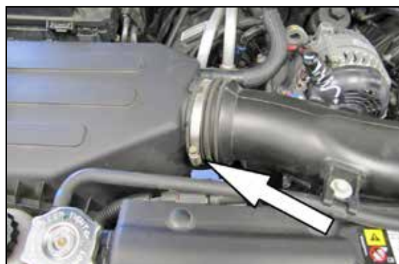
4. Loosen the hose clamp securing the factory intake tube to the air filter housing.
