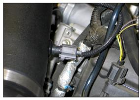
24. Connect the inlet air temperature sensor extension harness into the factory electrical connection and then connect the other end into the inlet air temperature sensor as shown.
