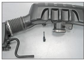
18. Release the locking tab and the remove the inlet air temperature sensor from the factory intake tube by twisting counter clockwise.
