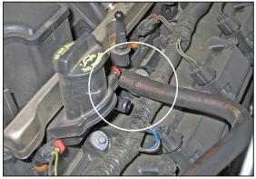
5. Disconnect the crankcase vent hose from the port on the valve cover.
