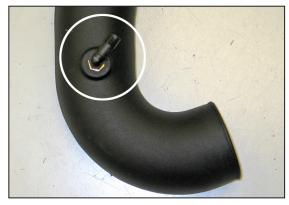
21. Install the 90° npt fitting into the K&N $^{\circ}$  intake tube as shown.
