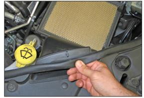
8. Unhook the sealing trim from the fresh air intake scoop.
