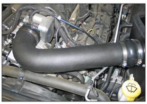
22. Install the K&N® intake tube into the silicone hump hose and then into the silicone hose at the throttle body, secure the intake tube with the provided hose clamp.
