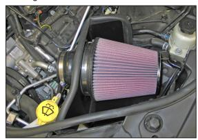
16. Install the K&N® filter onto the adapter and secure with the provided hose clamp.
