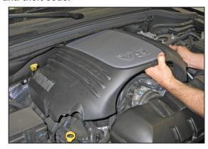
2. Lift up the engine cover to dislodge it from the mounting grommets and remove it from the vehicle.
