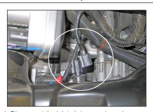
4. Disconnect the inlet air temperature air sensor electrical connection.
