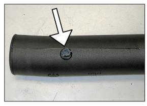
20. Install the inlet air temperature sensor into the  $K\&N^{@}$  intake tube.
