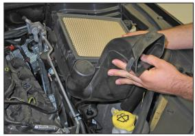
9. Lift up the lower airbox to dislodge it from the mounting grommets and then remove the lower airbox from the vehicle. Some vehicles may have a power steering line attached to the air box than will need to be unhooked.
