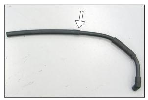
9. Install the provided silicone crank case vent hose onto the cut end of the factory crank case vent tube as shown.
