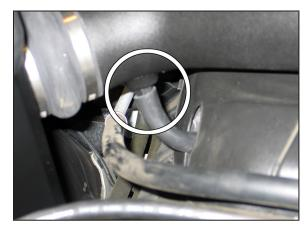
26. Connect the crank case vent hose to the vent fitting installed into the K&N® intake tube. Secure with the provided tie wrap.
