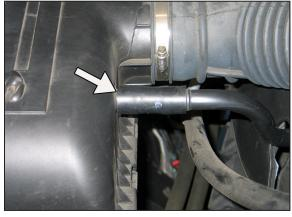
4. Disconnect the crank case vent hose from the air hox
