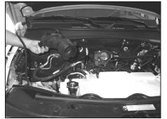
21. Remove the fresh air supply duct from the radiator core support as shown.
