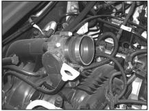
9. Install the silicone hose (084034) onto the throttle body and secure with the provided hose clamp.
