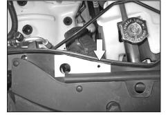
19. Using the provided template, place a mark onto the radiator core support for a hole to be drilled for the heat shield mounting bracket.
