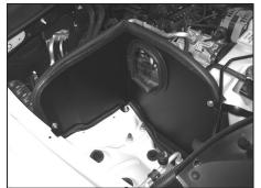
22. Install the heat shield assembly into the vehicle. Secure the rear of the heat shield to the mounting
