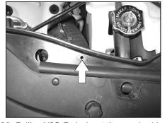
20. Drill a  $\frac{1}{4}$  O.D. hole at the marked location.
