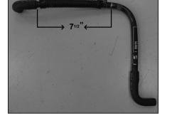
7. Using a knife, cut the crank case vent hose 7-1/2" from the valve cover elbow fitting as indicated.
