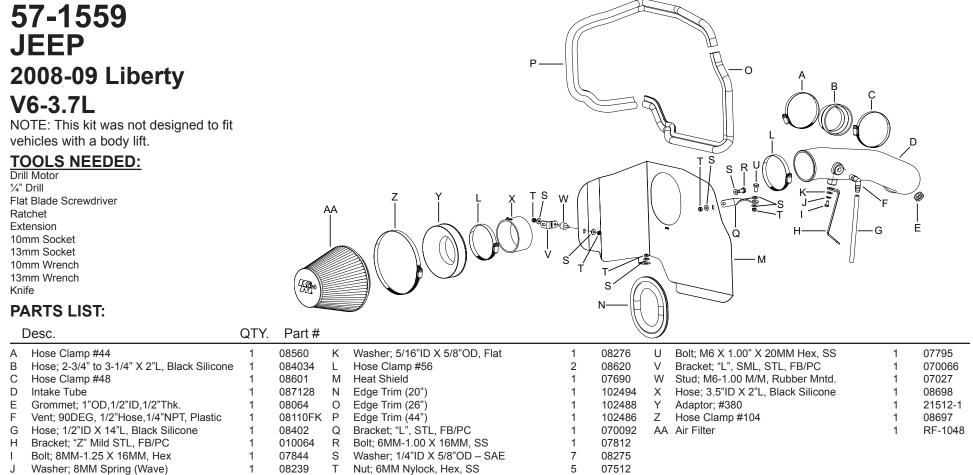
NOTE: FAILURE TO FOLLOW INSTALLATION INSTRUCTIONS AND NOT USING THE PROVIDED HARDWARE MAY DAMAGE THE INTAKE TUBE, THROTTLE BODY AND ENGINE.
