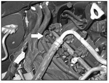
8. Reinstall the modified crank case vent tube onto the valve cover as shown.
