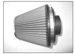
30. Install the filter adapter into the K&N air filter and secure with the provided hose clamp. NOTE: Drycharger<sup>®</sup> air filter wrap; part # RF-1048DK is available to purchase separately. To learn more about Drycharger<sup>®</sup> filter wraps or look up color availability please visit http://www.knfilters.com<sup>®</sup>.
