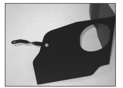
12. Secure the heat shield mounting bracket (070092) onto the heat shield as shown using the provided hardware.
