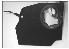
14. Install the provided edge trim into the hole of the heat shield as shown.
