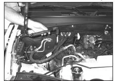
6. Remove the crank case vent tube assembly from the valve cover as shown.
