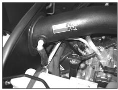
29. Connect the provided silicone vent hose to the modified factory vent tube and then connect the open end to the intake tube as shown.
