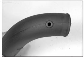
19. Install the provided grommet into the K&N^ ${\ensuremath{\mathbb{R}}}$  intake tube as shown.
