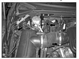
3. Disconnect the stock intake tube from the intake plenum. Lift to remove to remove the air box assembly from the vehicle as shown. 5. Lift to dislodge the intake plenum from it's mounting grommets and remove the intake plenum from the vehicle as shown.
