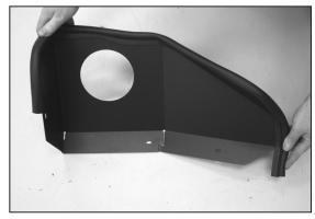
7. Install the provided edge trim onto the heat shield as shown. NOTE: Some trimming of the edge trim may be necessary.
