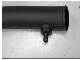
NOTE: Plastic NPT fittings are easy to cross thread. Install the vent fitting "hand" tight, then turn it two complete turns with a wrench.
