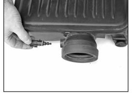
20. Twist the air temperature sensor counter clockwise and remove it from the stock intake plenum.
