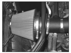
28. Install the air filter assembly onto the K&N<sup>(R)</sup> intake tube and secure with the provided hose clamp.
