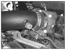
24. Reconnect the air temperature sensor electrical connection.
