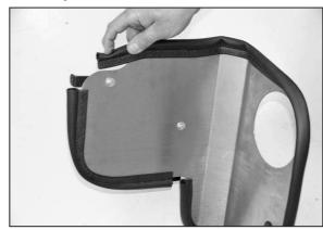
20. Install the long edge trim onto the heat shield assembly as shown.
