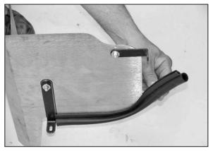
19. Install the short edge trim onto the heat shield assembly as shown.
