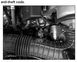
2. Release the red locking tab and disconnect the air temperature sensor electrical connection as shown.
