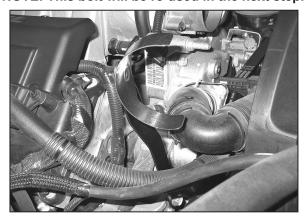
15. Install the tube mounting bracket assembly onto the upper alternator mount using the bolt removed in the previous step.
