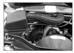
6. Remove the upper airbox housing and intake tube assembly as shown.
