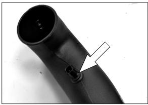
25. Install the air temperature sensor into the grommet installed into the K&N® intake tube in the previous step.
