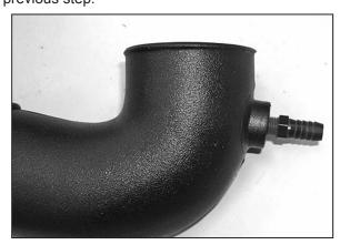
26. Install the 1/4" NPT fitting into the K&N® intake tube as shown.
