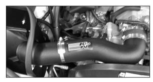
27. Install the K&N® intake tube into the silicone hose on the throttle body and align with the saddle clamp. Then, secure the intake tube with the provided hose clamps.
