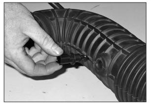
23. Remove the air temperature sensor from the stock intake tube as shown.
