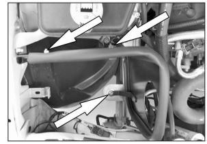
21. Install the heat shield assembly into the vehicle. Secure to the lower and upper airbox mounts and washer bottle stud with the provided hardware.
