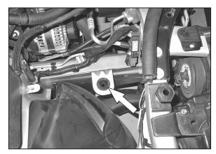
12. Remove the stock airbox mounting grommet as shown.
