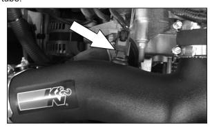
29. Re-connect the air temperature sensor electrical connection.
