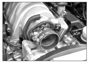
22. Install silicone hose (#08630) onto the throttle body and secure with the provided hose clamp.
