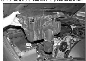
11. Lift the lower airbox, removing it from the vehicle as shown.
