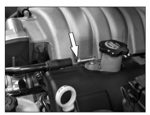
3. Disconnect the crankcase vent from the valve cover as shown.
