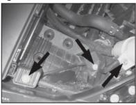
13. Remove the power steering reservoir mounting bolt and the two airbox bracket mounting bolts shown.
