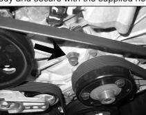
10. Remove the front engine bolt shown. **NOTE: This bolt will be reused.**
