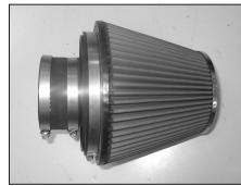
23. Install the silicone hose (08630) onto the air filter adapter and secure with the provided hose clamp.
