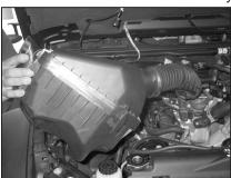
5. Lift up the airbox assembly to dislodge it from the mounting grommets and then remove the complete assembly from the vehicle.
