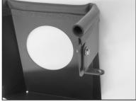
17. Install the supplied "L" bracket (070712) onto the heat shield as shown with the provided hard-
