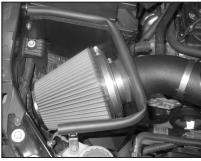
24. Install the K&N® air filter assembly on the intake tube and secure with the provided hose clamp as
