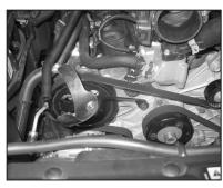
12. Install the tube mounting bracket assembly onto the engine and secure with the bolt removed in step #10.
