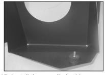
15. Install the supplied rubber mounted stud onto the heat shield with the provided hardware as shown.
