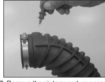
7. Remove the air temperature sensor from the stock intake tube as shown.
