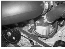
25. Reconnect the air temperature sensor electrical connection
