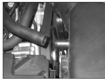
3. Disconnect the crankcase vent hose from the stock intake tube as shown.
