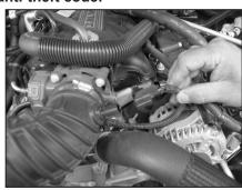
2. Release the locking tab on the air temperature sensor electrical connector and then disconnect the connection.
