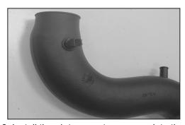
8. Install the air temperature sensor into the grommet installed into the intake tube during step #6. NOTE: Take care when handling the air temperature sensor as it is very fragile.
