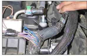
20. Place one washer onto the valve cover stud as shown.
