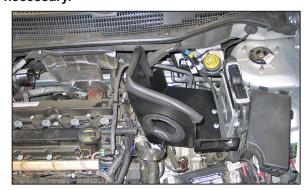
25. Install heat shield onto the mounting studs and secure with the two nuts removed in step #12 and the provided hardware.
