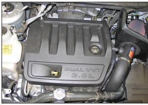
31. Reinstall the engine cover onto the engine.
