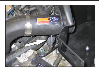
28. Reconnect the air temperature sensor electrical connection.
