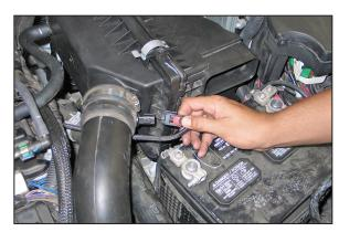
5. Depress the locking tab and disconnect the inlet air temperature sensor's electrical connection.
