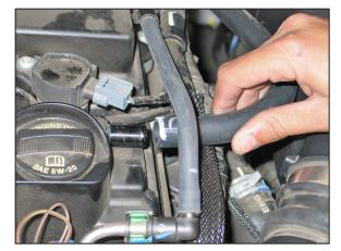
7. Disconnect the crankcase vent hose from valve cover.
