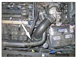
9. Loosen the hose clamp at the lower end of the stock intake tube from the vehicle.
