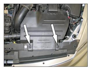
3. Rotate the fresh air tube fasteners counter clockwise to unlock them from the radiator core support.
