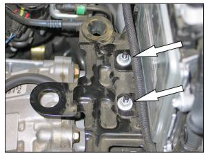
12. Remove the two airbox mounting nuts shown. **NOTE: These nuts will be reused in a later step.**
