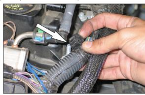
19. Unhook the wiring harness from the corner valve cover bolt as shown.
