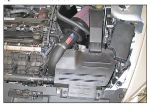
30. Install the fresh air duct into the heat shield and onto the core support. Then secure with the factory quarter turn fasteners.
