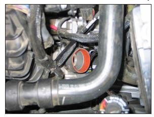
13. Install the silicone hose (08108) onto throttle body and secure with the provided hose clamp.
