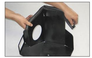
23. Install the long edge trim along the top of the heat shield as shown.
