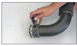
15. Remove the air temperature sensor from the factory intake tube as shown.
