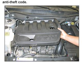
2. Pull up firmly to dislodge the engine cover from the mounting grommets. Then remove the engine cover from the vehicle.
