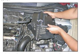
8. Pull up firmly to dislodge the airbox from the mounting grommets and then remove the airbox from the vehicle.
