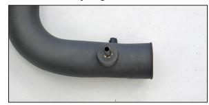
17. Install the supplied 1/4" npt vent fitting into the threaded boss in the K&N® intake tube as shown. NOTE: Plastic NPT fittings are easy to cross thread. Install the vent fitting "hand" tight, then turn it two complete turns with a wrench.
