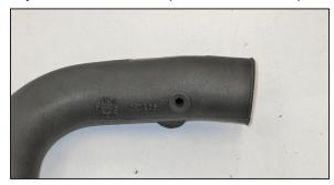
14. Install the supplied grommet into the intake tube as shown.
