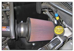
29. Install the K&N® air filter and secure with the provided hose clamp.
