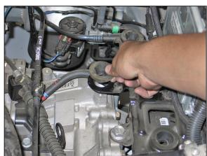
11. Remove the airbox mounting grommet shown.
