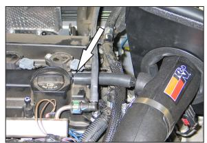
27. Install the provided crankcase vent hose onto the valve cover. Then onto the fitting installed into the K&N® intake tube.
