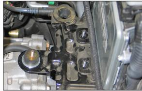
22. Install rubber mounted stud using the large fender washers provided.
