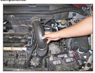
10. Remove the stock intake tube from the vehicle. NOTE: Be sure to unclip the wiring harness from the intake tube as you remove the tube from the vehicle.
