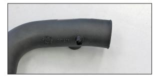
16. Install the air temperature sensor into the grommet.
