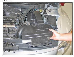
4. Remove the fresh air duct from the stock air filter housing and radiator core support.
