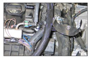
21. Install the tube mounting bracket assembly onto the valve cover stud and secure with the provided hardware.
