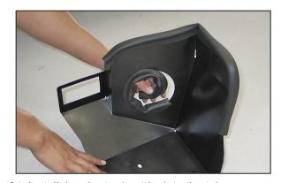
24. Install the short edge trim into the tube pass through hole as shown.
