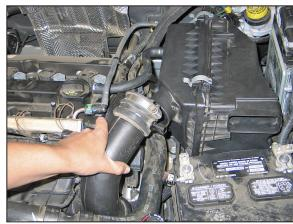
6. Loosen the hose clamp that secures the stock intake tube to the factory air filter housing.
