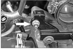
23. Remove the nut, which secures the intake plenum-mount shown.
