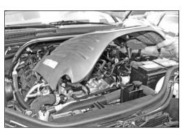
7. Remove the engine cover from the engine as shown.
