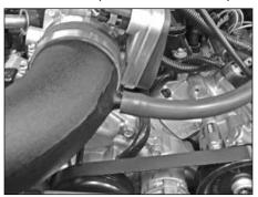
31. Install the provided crank case vent hose onto the valve cover and then onto the intake tube as shown.
