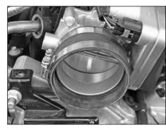
22. Install the silicone hose (08630) onto the throttle body and secure with the hose clamp provided.
