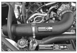
30. Install the intake tube into the silicone hose at the throttle body and onto the saddle clamp, then secure with the provided hose clamps.
