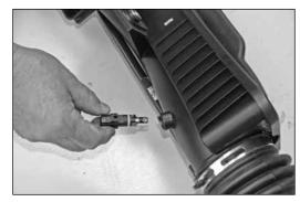
27. Rotate the air temperature sensor counter clockwise and remove the sensor from the stock intake plenum as shown.
