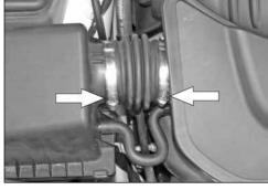
2. Loosen the hose clamp, which secures the stock intake tube to the intake plenum, and disconnect the crank case vent hose form the air box lid.
