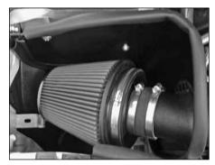
35. Install the K&N® air filter assembly onto the intake tube as shown and secure with the provided hose clamp.
