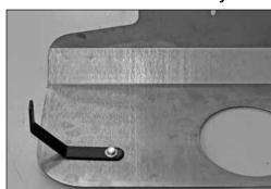
15. Install the supplied "C" bracket (07171) onto the heat shield as shown with the provided hardware. NOTE: Due to manufacturing tolerances, it may be necessary to us the provided spacer and longer bolt to attach the mounting bracket to the heat shield. This will enable the mounting bracket to align with the longer air box mounting brackets on some vehicles.
