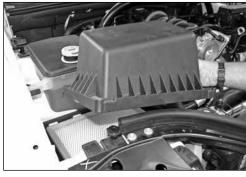
9. Un hook the air box lid retaining clamps and then remove air box lid and filter.
