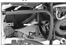
21. Install the heat shield assembly into the vehicle and secure to the lower and upper air box mounts and washer bottle stud with the provided hardware.
