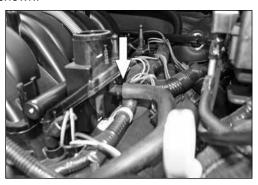
8. Remove the crank case vent hose from the engine as shown.
