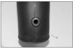
19. Install the provided grommet into the  $K\&N^{\mbox{\scriptsize \$}}$  intake tube as shown.
