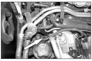
16. Install tube mounting bracket assembly onto A/C compressor using the bolt removed in step #14 as shown.
