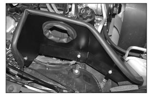
13. Install the heat shield assembly and secure with the provided hardware and the factory air box mounting nut.
