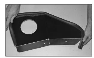
7. Install the provided edge trim onto the heat shield as shown. NOTE: Some trimming of the edge trim may be necessary.
