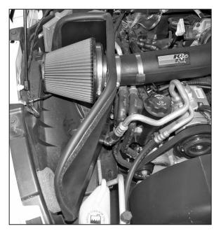
27. Install the Air filter assembly onto the K&N<sup>®</sup> intake tube and secure with the provided hose clamp as shown.
