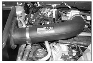
22. Install the K&N<sup>®</sup> intake tube onto the throttle body hose and position so the tube aligns with the saddle clamp. Secure with the provided hose clamps as shown.
