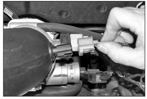
23. Reconnect the air temperature sensor electrical connection as shown.
