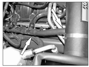
24. Install the provided silicone crank case vent hose onto the factory crank case vent tube and then onto the  $K\&N^{\mbox{\tiny \ensuremath{\mathbb{R}}}}$  intake tube as shown.
