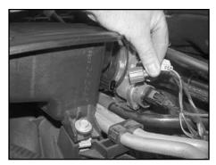
4. Depress the locking tab on the air temperature sensor electrical connection and then pull to disconnect he sensor electrical connection.
