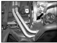
21. Remove the rear lower A/C mounting bolt shown.
