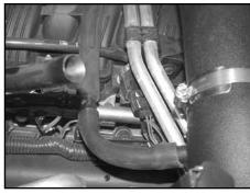
25. Install the provided crankcase vent hose onto the factory "Tee" fitting and then onto the K&N<sup>®</sup> intake tube as shown.
