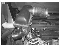
3. Disconnect the stock intake tube from the intake plenum and lift to remove the airbox assembly from the vehicle as shown.
