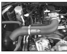
23. Install the K&N® intake tube into the silicone hose at the throttle body and onto the saddle clamp, then secure with the provided hose clamps.
