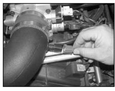
24. Reconnect the air temperature sensor electrical connection as shown.
