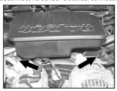
5. Loosen and remove the two intake plenum mounting bolts indicated
