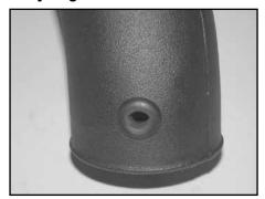
17. Install the provided grommet into the K&N<sup>®</sup> intake tube as shown.
