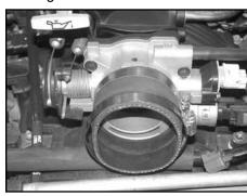
15. Install the silicone hose (08051) onto the throttle body and secure with the provided hose clamp as shown.
