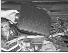
6. Lift and remove the intake plenum from the vehicle as shown.
