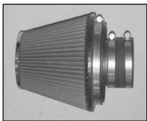
27. Install the silicone hose (08630) onto the air filter adapter and secure with the provided hose clamps as shown.
