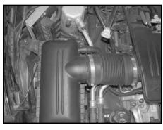
2. Loosen the hose clamp at the throttle body and the airbox mounting nut and then disconnect the crankcase vent hose from the "tee" fitting.
