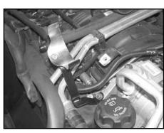
22. Using the bolt removed in step #21, install the tube mounting bracket onto the A/C compressor as shown.
