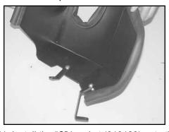
11. Install the "C" bracket (010123) onto the heat shield with the provided hardware as shown.
