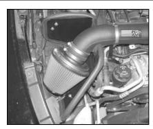
28. Install the air filter assembly onto the K&N<sup>®</sup> intake tube and secure with the provided hose clamp as shown.
