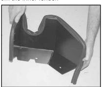
8. Install the provided edge trim onto the heat shield as shown.
