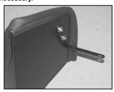
9. Install the "L" bracket (010124) onto the heat shield with the provided hardware as shown.
