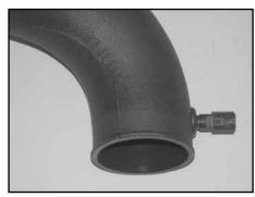
19. Install the sensor into the grommet installed in step #17.
