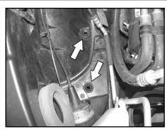
7. Pull the two airbox mounting grommets shown from the inner fender.
