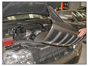
6. Remove the six grill retaining clips from the grill, then tilt the grill forward and lift to remove from the vehicle.
