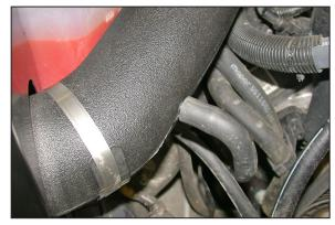
26. Connect the crankcase vent hose onto the  $K\&N^{\otimes}$  intake tube as shown.
