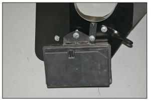
Using the provided spacer, install the vacuum reservoir onto the heat shield as shown.
