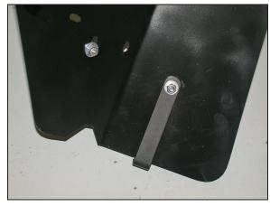
13. Install the "L" bracket (070952) onto the heat shield with provided hardware as shown. NOTE: Mount this bracket on the inside of the heat shield with the "L" pointing to the outside.
