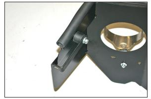
15. Install the bracket/rubber mounted stud assembly onto the heat shield as shown using the provided hardware.
