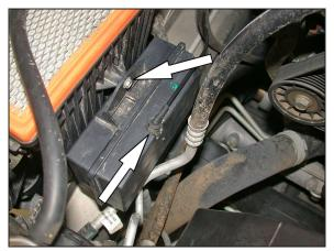
4. Disconnect the vacuum canister hose shown.
