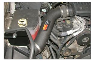
25. Install the K&N<sup>®</sup> intake tube into the silicone hose at the throttle body and onto the saddle clamp, then secure with the provided hose clamps as shown.
