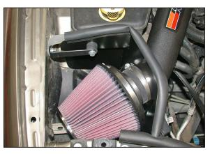
29. Install the air filter assembly onto the K&N<sup>®</sup> intake tube as shown and secure with the povided hose clamp.
