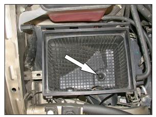
8. Remove the airbox mounting bolt shown.
