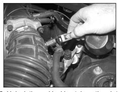
2. Unlock the red locking tab on the air temperature sensor electrical connection, then depress the locking lever and pull apart the temperature sensor electrical connection
