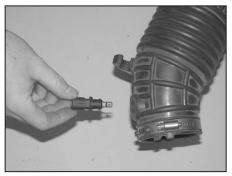
13. Remove the air temperature sensor from the factory intake tube.
