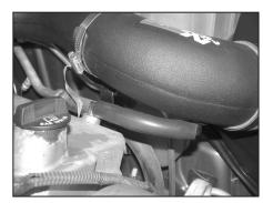
21. Install the provided silicone vent hose onto the valve cover vent and onto the elbow into the K&N intake tube as shown.
