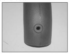
14. Install the provided grommet into the small throttle body end of the intake tube.
