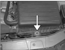
5. Loosen and remove the airbox mounting bolt as shown.
