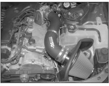
20. Install the K&N® intake assembly into the silicone hose at the throttle body and onto the saddle clamp as shown, then secure with the provided hose clamps. Adjust the air filter assembly for best clearance and tighten the hose clamp, which secures it to the K&N® intake tube.
