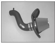
18. Install the air filter assembly onto the K&N<sup>®</sup> intake tube as shown.
