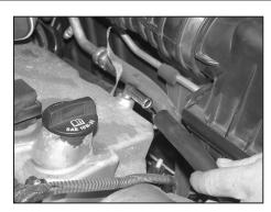
4. Disconnect the crankcase vent hose from the valve cover port as shown.
