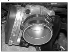
19. Install the silicone hose (08190) onto the throttle body and secure with the provided hose clamp as shown.
