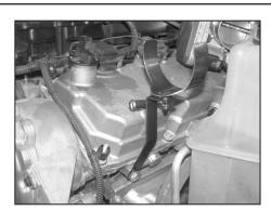
8. Using the provided hardware, install the tubemounting bracket onto the engine at the threaded hole in the cylinder head as shown.
