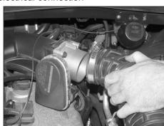
3. Loosen the hose clamp that secures the intake tube to the throttle body and pull the intake tube off the throttle body.
