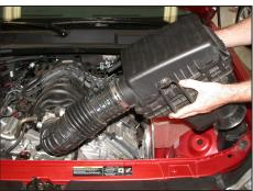
7. Lift the complete intake and air filter assembly to remove it from the vehicle.
