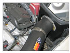
19a. On SRT 8; 6.1L equipped vehicles, connect the factory crank case vent hose onto the 90° fitting installed into the K&N® intake tube (in step #16c).
