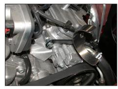
13. Using the provided spacer, install the tube mounting bracket assembly onto the engine as shown.
