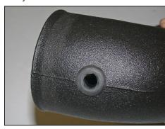
16. Install the provided grommet into the K&N® intake tube as shown.
