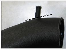
16a. On SRT 8; 6.1L vehicles, cut the vent off of the  $K\&N^{\odot}$  intake tube as shown.
