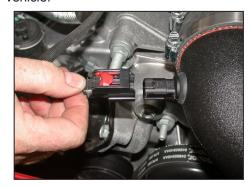
3. Unlock the red locking tab on the air temperature sensor electrical connection, then depress the locking lever and pull apart the temperature sensor electrical connection.
