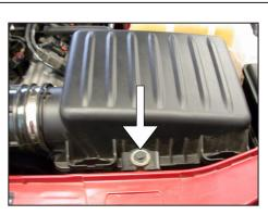
6. Loosen and remove the air box mounting bolt as shown.
