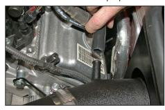
19. Install the provided crank case vent hose onto the vent port on the valve cover then install the vent hose onto the K&N® intake tube.
