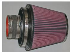
21. Install silicone hose (08630) onto the air filter assembly and secure with the provided hose clamp.
