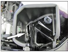
11a. Due to vehicle manufacturing tolerances, the A/C lines on some vehicles may need to repositioned slightly so that they do not contact the heat shield. To adjust, grab the A/C line on the aluminum section and carefully apply pressure in the desired direction until clearance is obtained.
