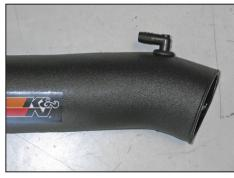
16d. On SRT 8; 6.1L equipped vehicles, install the provided 90° hose mender as shown.
