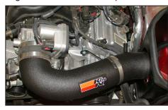
18. Install the K&N® intake tube into the throttle body and onto the saddle clamp as shown, then secure with the hose clamps provided.
