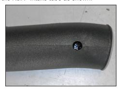
16b. Drill out the hole in the intake tube to 0.75".
