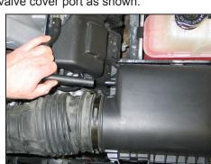
5a. On SRT-8; 6.1L vehicles, disconnect the crank case vent hose from the air box as shown.
