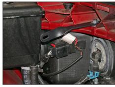
8. Install the twist bracket (070772) onto the core support using the hardware provided through the existing hole as shown.
