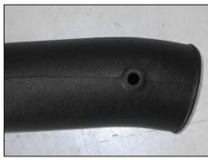
16c. On SRT 8; 6.1L equipped vehicles, install the provided grommet into the 0.75" ID hole as shown.
