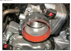
14. Install the silicone hose (08630) onto the throttle body and secure with the provided hose clamp as shown.
