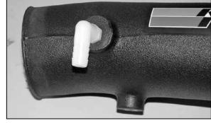
22. Install the 90° NPT fitting into the K&N $^{\! \rm 8}$  intake tube as shown.
