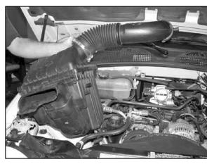
5. Firmly lift up to disengage the airbox from the retaining grommets and remove the airbox from the
