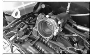
18a. On 2007 vehicles with a plastic throttle body, install the supplied silicone hose (084034) onto the throttle body and secure with the provided hose clamps as shown.
