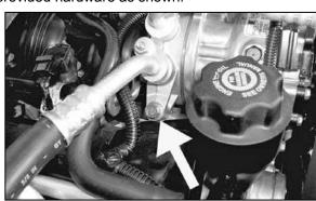
17. Remove the A/C compressor-mounting bolt.
