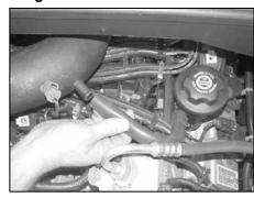
25. Connect the provided silicone hose to the crank case vent on the valve cover, then connect to the K&N® intake tube.
