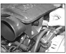
7. Depress the locking tab on the air temp sensor and disconnect its electrical connection.
