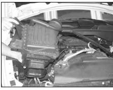
5. Pull up firmly to dislodge the air box from the mounting grommet, and remove the air box from the vehicle.
