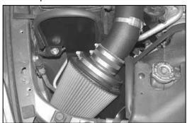
28. Install the K&N® air filter assembly onto the K&N® intake tube and secure with the provided hose clamp.
