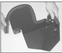
13. Install the provided edge trim onto the heat shield. Trim if necessary.
