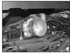
17. Install the silicone hose (08630) onto the throttle body and secure with the provided hose clamp.
