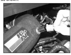
24. Reconnect the temp sensor electrical connection.
