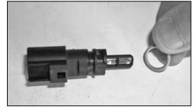
19. Remove the O-ring from the air temp sensor as shown.
