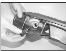
18. Twist the temp sensor counter clockwise to unlock and remove the temp sensor from the resonator.
