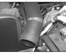
23. Using the provided hose clamp, secure the  $K\&N^{\circ}$  intake tube to the saddle bracket assembly as shown.
