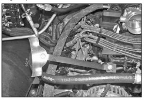
21a. On vehicles equipped with an air injection valve, secure the tube mounting bracket assembly (#07192) to the resonator mount on the intake manifold. Secure using the provided 6mm hardware as shown.
