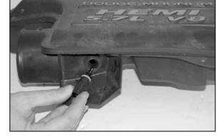
23. Twist the temp sensor counter clock wise to remove from the resonator box as shown.
