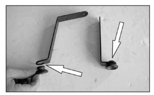
10. Install the two rubber bushings that were removed in the previous step into the provided brackets as shown.
