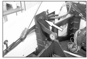
18. Install the twisted "L" bracket with the bolt that was removed in step 17. Do not tighten bolt completely.
