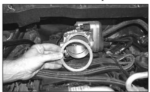
2. Loosen the hose clamp that connects the intake tube to the resonator box then remove the intake tube.
