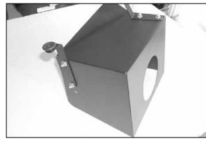
12. Install the "L" bracket onto the heat shield with the provided hardware. Do not tighten completely at this time.
