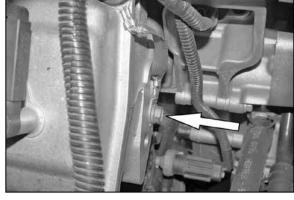
20. On vehicles not equipped with an air injection valve, remove the bolt that secures the ground strap shown.
