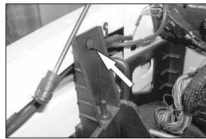
17. Remove the 8mm bolt that retains the airbox mount.
