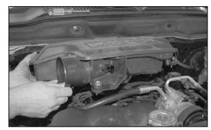
7. Remove the resonator box from vehicle. NOTE: K&N Engineering, Inc., recommends that customers do not discard factory air intake.
