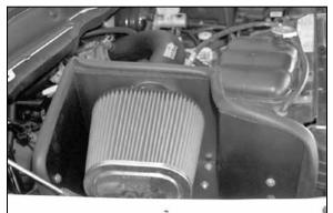
32. Install the K&N $^{\ensuremath{\circledast}}$  air filter onto the intake tube as shown.
