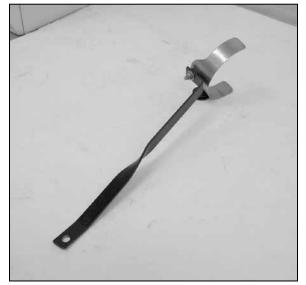
19. On vehicles that are not equipped with an air injection valve, assemble the tube mounting bracket (#07161) and saddle clamp as shown.
