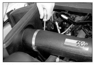
29. Using the provided hose clamp, secure the  $K\&N^{\mbox{\tiny @}}$  intake tube to the saddle bracket assembly as shown.
