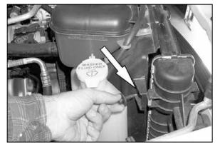
15. Remove the 13mm bolt from the upper fan shroud as shown.
