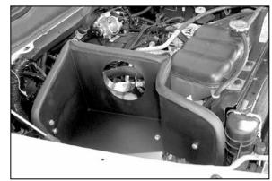
22. Install the heat shield onto the factory airbox studs then mount to the previously installed brackets.
