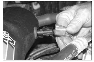
31. Reconnect the air temp electrical connection.
