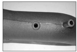
25. Install the provided grommet into the intake tube as shown.
