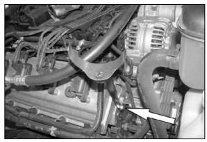
21. On vehicles not equipped with an air injection valve, install the tube mounting bracket assembly (#07161) onto the cylinder head, along with the ground strap removed in the previous step. Secure using the provided 8mm hardware.
