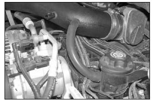
30. Connect the provided vent hose onto the oil fill then onto the new intake tube as shown.
