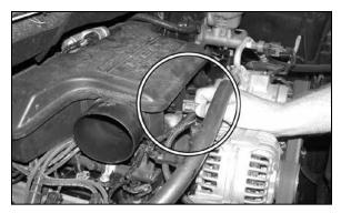
4. Disconnect the air temp sensor electrical connection as shown.
