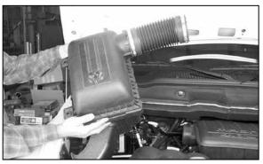
3. Lift up firmly to release the airbox from mounting studs, then remove completely.
