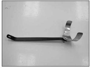
19a. On vehicles equipped with an air injection valve, assemble the tube mounting bracket (#07192) and saddle clamp as shown.
