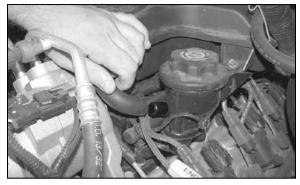
6. Disconnect the crankcase vent hose from oil fill as shown.
