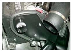
24. Install the K&N $^{\mbox{\tiny B}}$  air filter onto the air temperature sensor as shown.
