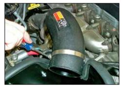
22. Install the intake tube onto the turbo inlet, then align with the saddle bracket. Attach the saddle bracket to the intake tube with the provided hose clamp, adjust the bracket to achieve the appropriate clearance for the intake tube before tightening.
