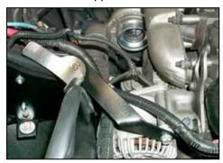
19. Install the saddle bracket assembly onto the alternator with the bolt that was removed in the previous step.
