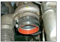
20. Install the silicone hose (08761) onto the turbo with the provided hose clamp.
