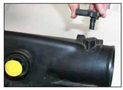
11. Remove the temperature sensor from the air box lid using an 9/32 socket.
