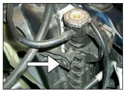
13. Remove the bolt that retains the fan shroud to the radiator.
