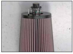
23. Install the grommet and air filter minder that was removed in step 21 onto the  $K\&N^{\ensuremath{\circledast}}$  air filter as shown.
