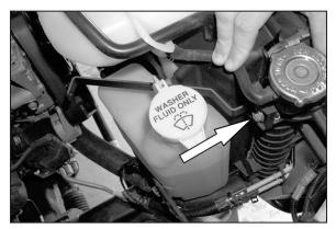
13. Install the provided bracket onto the radiator shroud with the provided 8mm bolt and washers. **NOTE: Do not tighten completely.**
