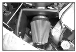
30. Install the air filter assembly onto the intake tube and adjust for maximum clearance around the filter.
