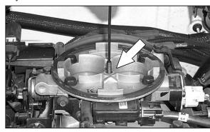
24. Install the provided stud into the throttle body as shown.
