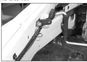
15. Install the provided L bracket onto the inner fender well with the bolt that was removed in step 14.
