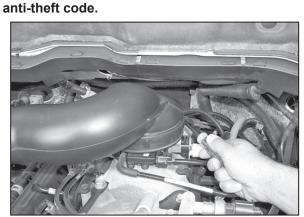
2. Loosen the hose clamp on the air intake tube at the throttle body.
