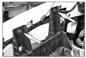
9. Use a 13mm wrench to remove the two bolts that retain the upper airbox mount.
