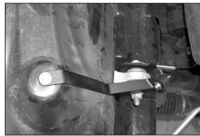
17. Install bracket and bumper stud onto inner fender well with hardware provided.
