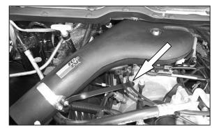
27. Secure the saddle bracket to the intake tube with the provided hose clamp as shown. Then tighten the bolt at the fuel rail (see arrow). Position the heat shield for best fit and clearance.
