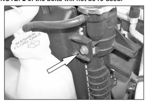
12. Remove the upper radiator shroud bolt.
