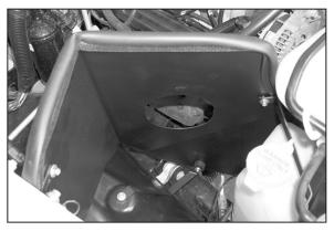
19. Install heat shield onto the vehicle with the provided hardware.
