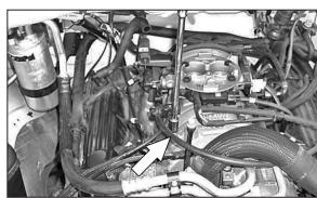
21. Using a 1/2" socket, loosen and remove the bolt that retains the fuel rail bracket.
