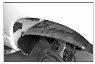
7. Remove the 8 bolts that retain the inner fender to the vehicle. To allow inner fender well to drop for access to the lower airbox mount bolts.
