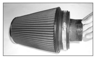
28. Install filter onto the radius filter adapter as shown.
