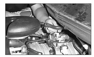
25. Attach the crankcase vent hose assembly to the vent tube on the intake tube.
