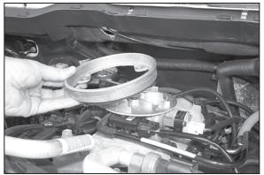
6. Remove the throttle body adapter and factory gasket from throttle body. Then re-install and tighten the 4 bolts that were removed in step 5.
