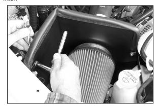
31. Align the heat shield for best clearance then tighten the 3 brackets.
