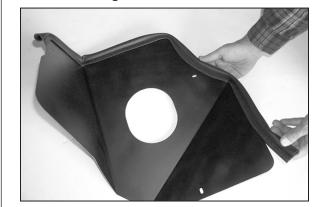
18. Install edge trim onto heat shield as shown. Trim if needed.
