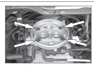
5. Using a 1/2" socket, remove the 4 bolts that retain the throttle body adapter.
