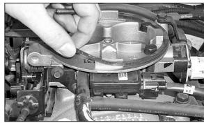
23. Apply the new provided gasket on the throttle body as shown.
