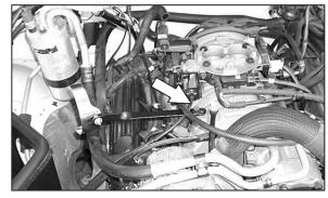
22. Install the saddle bracket assembly using the bolt removed in step #21.
