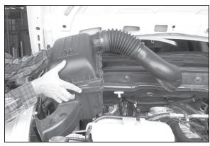
4. Lift up firmly to release the airbox from mounting studs, then remove completely.
