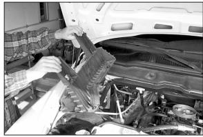
10. Remove the airbox mount as shown.
