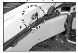
14. Using a 10mm wrench remove the bolt from the inner fender well.
