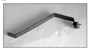
16. Install the provided rubber mounted stud onto the bracket as shown.
