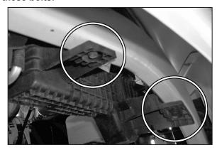
8. Use a 13mm wrench to remove the two bolts that retain the lower airbox mount.
