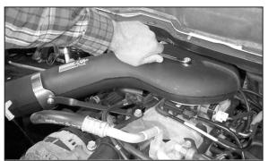
26. Install the intake tube onto the throttle body and secure the plenum with the provided nut extension and washer.
