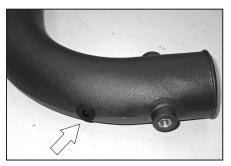
25. Install the provided grommet into the K&N $^{\mbox{\tiny \$}}$  intake tube as shown.
