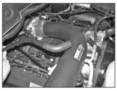
30b. On models that the crank case vent hose is connected to the passenger side valve cover, remove the factory 90° coupling hose from the plastic vent tube.
