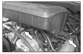
6. Pull up firmly to release the resonator from engine.
