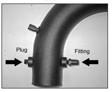
27b. On 2008 and later model year vehicles, install the NPT fitting and NPT plug as shown.
