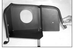
14. Install the provided edge trim onto the heat shield. Trim if necessary.
