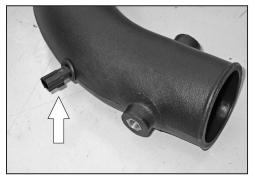
27. Install the air temp sensor into the  $K\&N^{\ensuremath{\$}}$  intake tube as shown.
