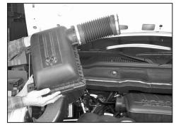
3. Lift up firmly to release the air box from mounting studs, then remove completely.
