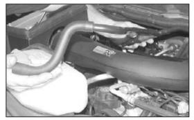
30a. On models that the crank case vent hose is connected to the "T" on the passengers side of the engine, remove the complete vent tube assembly from the rubber fittings in each valve cover as shown.
