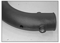
24. On models that come equipped with temp sensors, drill a 7/8" hole in the K&N $^{\odot}$  intake tube at the drill point.
