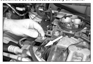
5. Remove the stock grommet and the stock plastic locating pin as shown.
