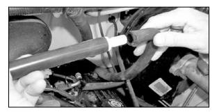
33. Assemble the provided hose mender and the provided silicone hose as shown, then connect it to the stock crank case vent hose as shown.
