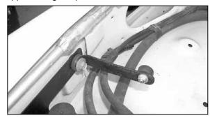
22. Secure the "L" bracket to the EVAP assembly bracket using the existing bolt as shown.
