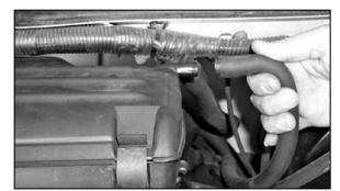
3. Disconnect the crank case vent hose as shown.
