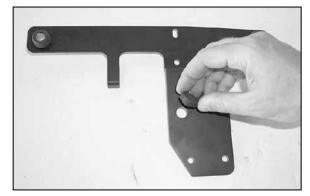
12. Install the provided step bushing into the hole on the backside of the K&N® EVAP assembly bracket as shown.
