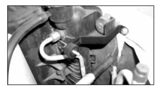
21. Secure the "Z" bracket to the radiator core support using the provided hardware as shown.
