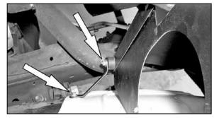
27. Install the bracket onto the inner fender using the provided hardware as shown, then, secure the rubber mounted stud to the bottom of the heat shield halves and secure with the provided hardware as shown.
