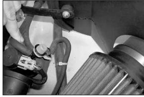
40. Using the provided zip tie, bundle up the EVAP assembly vent hoses as shown.
