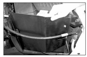
24. Install the first half of the heat shield into the vehicle and secure it to the "Z" bracket using the provided hardware as shown.
