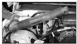
2. Remove the air inlet duct as shown.
