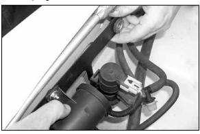
16. Install the purge control solenoid onto the K&N<sup>®</sup> EVAP assembly bracket as shown.
