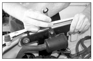
14. Install the EVAP canister vent onto the EVAP assembly bracket using the hardware provided as shown.
