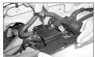
13. Install the EVAP canister onto the K&N® EVAP assembly bracket using the original screws removed in step 9.
