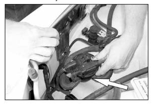
9. Loosen and remove the three screws that secure the EVAP canister to EVAP assembly bracket as shown.
