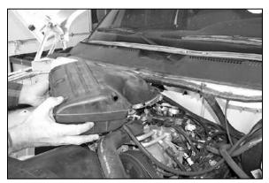
4. Loosen the hose clamp at the throttle body, then, remove the air cleaner assembly by pulling firmly upwards as shown.
