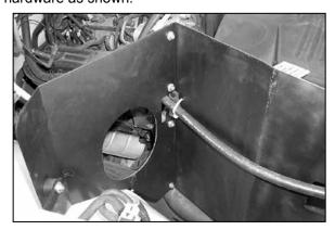
28. Secure the two heat shield pieces using the provided hardware as shown, then, secure the A/C hard line to the heat shield using the provided zip tie as shown.
