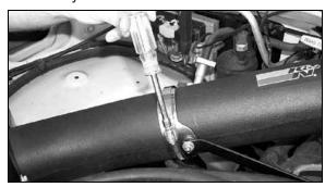
37. Secure the K&N® intake tube to the saddle bracket using the provided hose clamp as shown.
