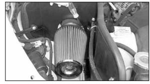
39. Install the K&N® Air Filter onto the K&N® intake tube and secure it with the provided hose clamp as
