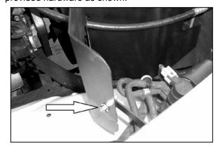
25. Install the second half of the heat shield into the vehicle and secure it to the "L" bracket using the provided hardware as shown.
