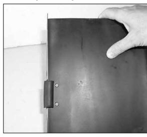
23. Install the provided edge trim onto the cut-out on the heat shield as shown.
