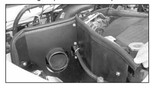
38. Install the provided edge trim onto the K&N® heat shield as shown.
