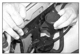
8. Loosen and remove the EVAP canister vent from the EVAP assembly bracket as shown.
