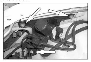
7. Loosen and remove the three bolts that secure the EVAP assembly bracket to the inner fender as shown.
