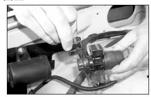
15. Remove the rubber mounted locating bracket from the purge control solenoid as shown.
