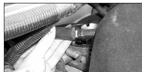
34. Connect the silicone hose to the crank case vent on the K&N® intake tube as shown.
