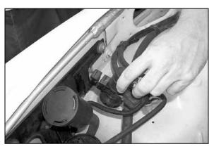
6. Remove the EVAP canister purge solenoid from the EVAP assembly bracket located on the inner fender as shown.
