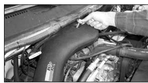
35. Install the nut extension and the provided washers into the hole on the K&N® intake tube as shown.
