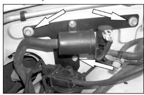
17. Using the two stock bolts and the provided sheet metal screw, secure the EVAP assembly bracket to the inner fender as shown.
