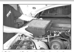
4. Pull upward firmly on the airbox base to release it from it's mounting studs and remove. NOTE: K&N Engineering, Inc., recommends that
