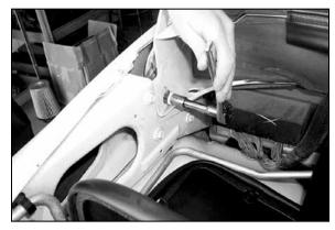
15. Loosen and remove the bolt that retains the hood hinge to the inner fender and remove hood hinge bolt from vehicle.
