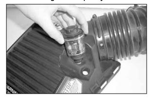
13. Remove the filter restriction gauge and grommet from the stock airbox as shown. NOTE: Use caution when removing gauge.
