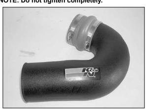
9. Attach the hump hose onto the K&N® intake tube as shown.
