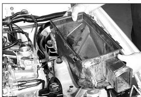
6. Remove the lower air cleaner assembly as shown
