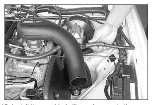
15. Install the provided silicone hose onto the EVAP canister vent line then secure the other end onto the K&N® intake tube.
