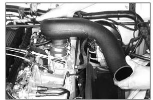
13. Install the K&N® intake tube onto the throttle body and tighten the hose clamp.
