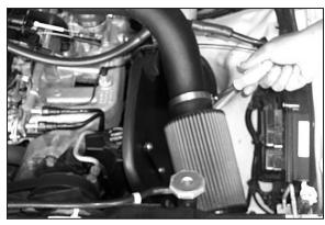
16. Install the K&N® Filtercharger onto the K&N® intake tube as shown.
