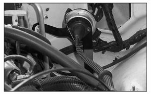
19. Using one of the nuts removed in step #8, and the bolt removed in step #12, secure the cruise control assembly as shown.
