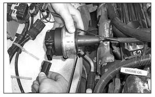
8. Loosen and remove the three nuts that secure the cruise control bracket, then pull the cruise control assembly upwards to disconnect the cruise control electrical connection as shown.
