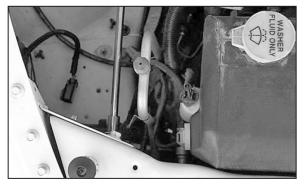
12. Loosen and remove the bolt that secures the inner fender to the radiator core support.
