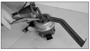
13. Loosen and remove the two nuts that secure the cruise control actuator to the bracket, then slide the diaphragm cover upwards and remove the pin from the cable end.
