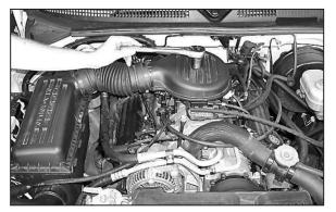
2. Loosen and remove the plenum retaining nut.
