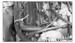
27. Using one of the provided zip ties, secure the A/C line and heater hose together as shown. **NOTE: when installing the K&N® intake tube, check the two hoses for clearance under the intake tube and adjust for best fit.**
