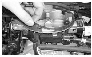
31. Apply the new provided gasket on the throttle body as shown.
