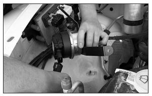
18. Position the cruise control into the vehicle in order to reconnect the cruise control electrical connection as shown.
