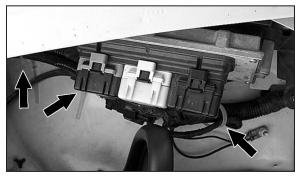
36. Using the provided zip-ties, secure the wire harness as shown.
