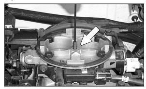
32. Install the provided stud into the throttle body as shown.
