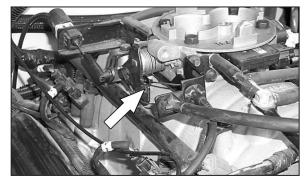
26. Slide the cruise control cable through the cable retainer and clip in place, then reconnect the cable end onto the the throttle post as shown.
