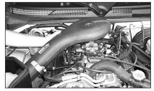
33. Slide the K&N<sup>®</sup> intake tube through the hole in the heat shield as shown.
