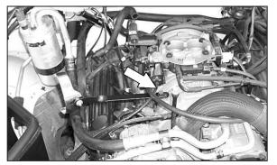
30. Install the saddle bracket assembly using the bolt removed in step #28. **DO NOT TIGHTEN COMPLETELY.**
