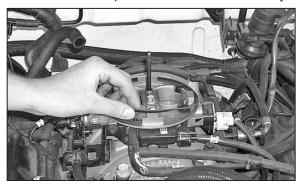
10. Remove the throttle body gasket as shown.
