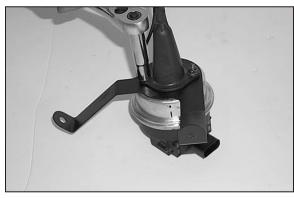
16. Using the original nuts secure the cover to the cruise control assembly, as shown.
