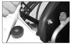
24. Attach the "C" bracket to the inner fender flange with the hardware provided as shown. **DO NOT TIGHTEN COMPLETELY.**
