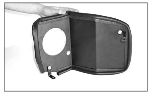
21. Secure the "L" and "C" brackets to the heat shield with the hardware provided as shown. **DO NOT TIGHTEN COMPLETELY.**
