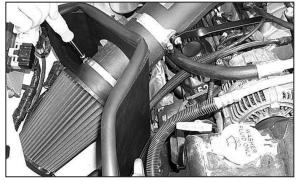
37. Install the K&N<sup>®</sup> Air Filter and secure with the provided hose clamp.
