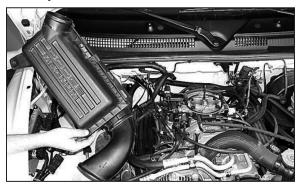
4. Loosen and remove the nut that secures the air box to the inner fender, then pull firmly upward to release the air box from its mounting grommets and remove the air box assembly. **NOTE: K&N recommends that you do not discard your factory air intake.**  5. Remove the cruise control vacuum line from the vacuum tee on the firewall.
