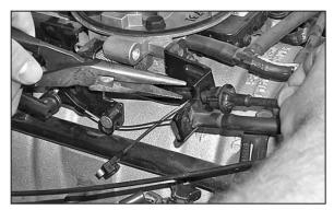
7. Using a pair of pliers, squeeze the release tabs on the cruise control cable, then pull the cable out of the retaining bracket.
