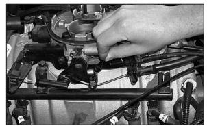
6. Remove the cruise control cable at the throttle body.
