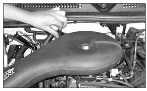
38. Reconnect the crankcase vent line to the K&N<sup>®</sup> intake tube as shown.
