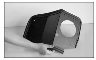
20. Apply the edge trim to the heat shield and trim to fit as shown.
