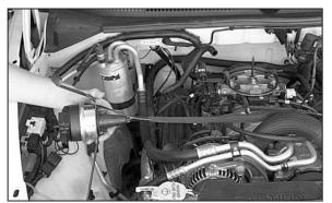
9. Remove the complete cruise control assembly.
