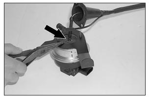
15. Slide the cable end back onto the actuator shaft and reinstall the pin as shown.
