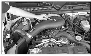
34. Install the K&N<sup>®</sup> intake tube onto the throttle body and secure the plenum with the provided nut extension, and washer.
