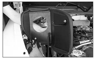
22. Position the heat shield into the vehicle and feed the cruise control cable and vacuum line through the small hole in the heat shield, then place the grommet into the hole in the heat shield.
