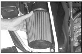
24. Install the K&N® air filter element onto the intake tube and tighten with the provided hose clamp.
