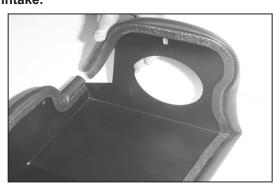
9. Install trim seal onto the heat shield.
