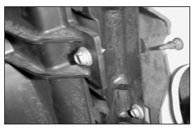
11. Loosen and remove the upper radiator shroud's retaining bolt.
