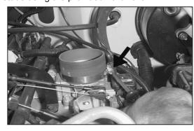
18. Attach the silicone hose to the throttle body using the provided hose clamp.
