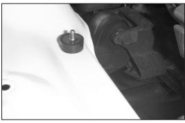
13. Install the second rubber mount stud into the lower air box mounting point using the provided hardware.
