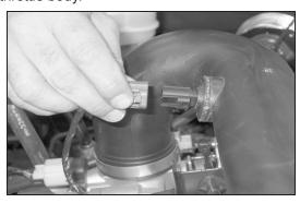
3a. On vehicles equipped with a temperature sensor, depress the temperature sensor electrical connection locking tab and then pull on the connector to disconnect the connection.
