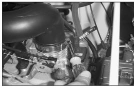
3. Loosen the hose clamp on the intake tube at the throttle body.
