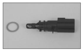
5a. Remove the sealing o-ring from the temperature sensor as shown.
