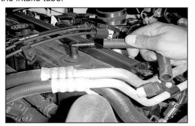
22. Detach the crank case vent hose from the vent fitting on the valve cover.
