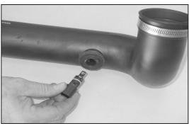
5. On vehicles equipped a with temperature sensor, lift the temperature sensor-locking tab while twisting the sensor counter clockwise to remove the sensor from the intake tube.
