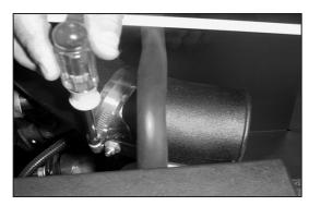
20. Secure the intake tube to the saddle bracket using the provided hose clamp.
