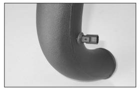
19c. Install the temperature sensor into the grommet as shown.
