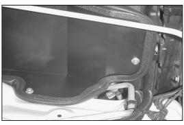
17. Secure the heat shield to the rubber mount studs using the provided hardware.
