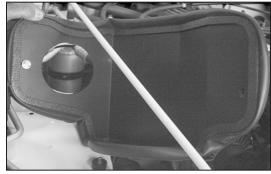
16. Install the heat shield assembly.
