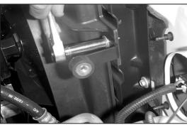
12.Install the "L" bracket using the bolt removed in the previous step.
