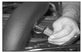
23a. Reconnect the temperature sensor electrical connection to the temperature sensor.
