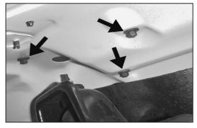
7. Loosen and remove the 3 nuts that retain the air box base to the inner fender apron.
