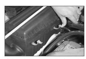
4. Release the 5 over center clips that retain the air box top to the air box base.
