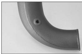
19b. Remove the K&N $^{\circ}$  intake tube from the vehicle and drill a 3/4" hole at the position marked in step #19a. Install the provided grommet into the hole that was drilled out.
