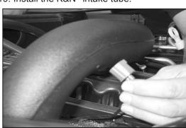
19a. Position the temperature sensor electrical connector next to the  $K\&N^{\otimes}$  intake tube for the best fit, then mark the location to be drilled.
