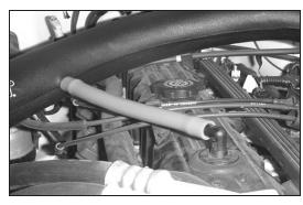
23. Attach the provided vent hose onto the vent fitting of the valve cover and the K&N® intake tube.
