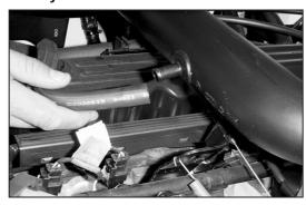
2. Detach the crank case vent hose from the stock intake tube.
