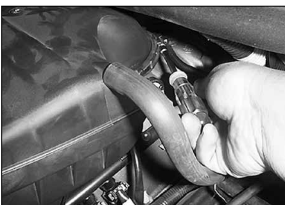
2. Loosen the hose clamp on the air cleaner at the throttle body.
