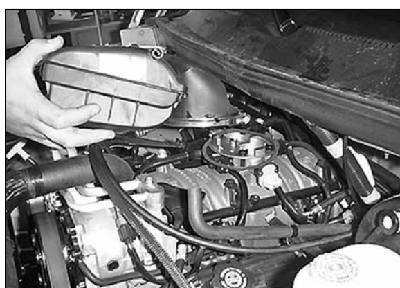
4. Pull firmly upwards to remove the air cleaner away from the throttle body.
