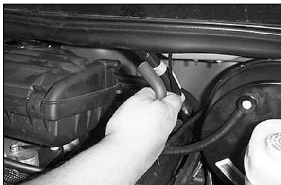
3. Disconnect the crankcase vent line from the air cleaner.
