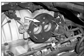
11. Install adapter base plate as shown. NOTE: The location of the idle air hole, if installed upside down vehicle will not run.
