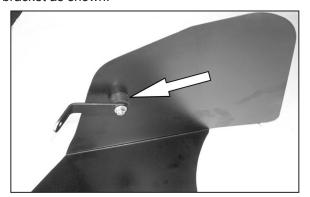
21. Install the new "L" bracket onto heat shield as shown.
