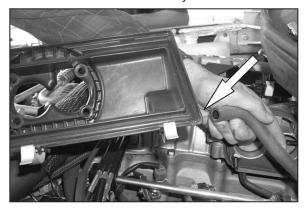
6. Disconnect crank case vent from air box base as shown. Then remove air box from vehicle.
