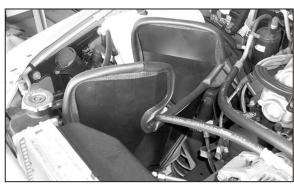
26. Install heat shield onto vehicle then mount using hardware provided.
