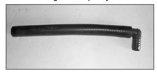
32. On vehicles that come equipped with an air injection pump, install the 90 degree fitting into the vent line as shown.
