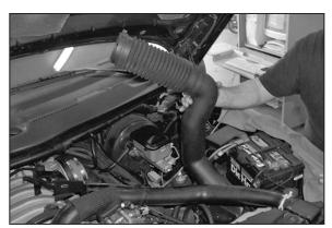
3. Unbolt the 10mm bolt at the bottom of fresh air intake tube then remove complete intake tube from vehicle.
