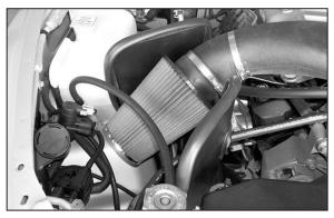
34. Install the K&N Air Filter onto the new K&N® intake tube as shown.
