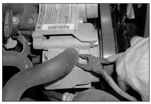
15. On vehicles that come equipped with an air injection pump, release spring clamp that secures the air pump intake hose.
