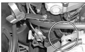
28. Install the new bracket behind alternator and secure with the nut that was removed in previous step.
