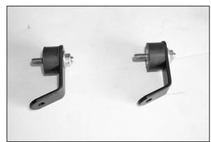
17. Assemble the two rubber mounted studs onto the two "L" brackets as shown.
