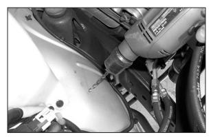
24. Remove heat shield assembly, then drill a ¼" hole on the spot previously marked.
