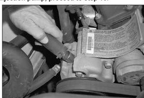
15a. Remove the intake hose from air pump as shown.
