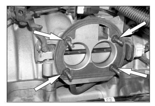
7. Loosen and remove the 4 11mm nuts that retain the throttle body to intake manifold.
