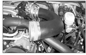
30. Install the new K&N® intake tube onto throttle body as shown.
