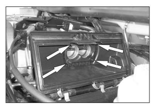
5. Loosen and remove the 4mm nuts that retain the air box base to the throttle body.
