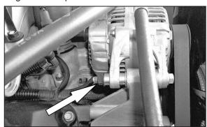
27. Remove nut that retains alternator onto factory bracket.
