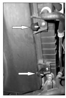
19. Install the two brackets onto the fan shroud with the bolts that were removed in the previous step.
