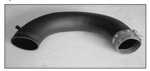
29. Install the provided silicone hose approximately half the length of the silicone hose onto the new K&N® intake tube as shown.
