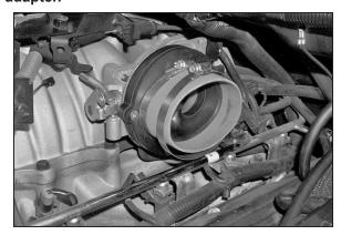
14. Install the provided silicone hose onto the throttle body adapter with the provided hose clamp.
