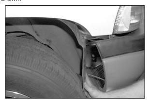
15b. Remove the 3 inner fender mounting retainers by pushing the center release pin in with an 1/8"
