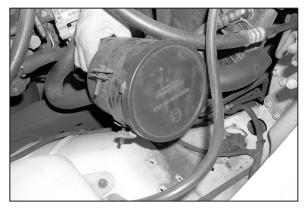
15d. Remove the three 7/16" nuts that retain the air pump muffler. Then pull up to remove the mounting studs from inner fender apron.
