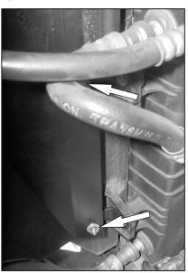
22. Install the heat shield assemble onto the vehicle and secure it to the rubber mounted studs using the provided hardware as shown.
