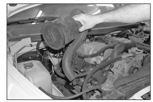
15e. Remove muffler and intake hose assembly from vehicle.
