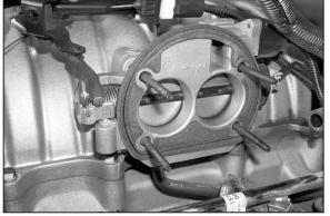
9. Remove throttle body gasket from throttle body.
