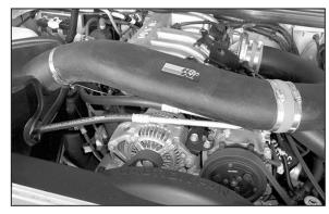
31.Install the second intake tube into silicone hose and then secure the intake tube to saddle bracket. **NOTE: Do not tighten completely.**
