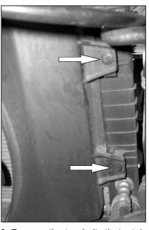
18. Remove the two bolts that retain the fan shroud to the radiator as shown.
