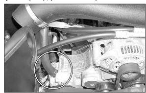
32a. Connect the silicone hose onto the air pump with the provided hose clamp as shown.
