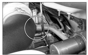
33. Reconnect the crank case vent onto the new K&N® intake tube as shown. Trim vent hose for best fit.
