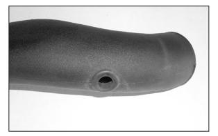
32c. Use a 1-1/4" hole saw and drill a hole where the intake tube was marked in the previous step. Then install the provided grommet as shown.
