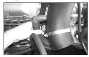
32b. Mark the intake tube where the 90 degree fitting lines up with the intake tube then remove the intake tube from vehicle
