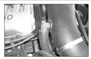
32d. Re-install the intake tube onto the vehicle then install the 90 degree fitting into the grommet on the intake tube as shown.
