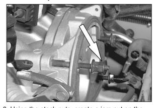
8. Using the stock nuts, create a jam nut on the stock stud and loosen the 4 studs. NOTE: Do not remove studs at this time.
