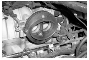
13. Install the provided gasket and throttle body top plate with the provided hardware. Then torque to 30 inch pounds.
