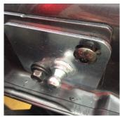
Tighten the button head with an M5 allen wrench and the other bolt with a 10mm wrench.
