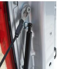
Periodically check the upper and lower mounting locations to insure that parts have not loosened through repeated use. If either mounting location is found to be loose, re-tighten the hardware as needed.
