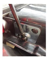
Install the cable back onto the cable bolt, and the larger part of the shock on the ball mount.
