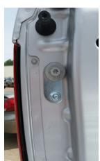
Tighten the bolt with the T50.
