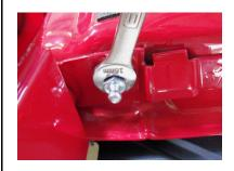
Using a torque wrench to install the ball mount will also insure that the blind nut has been completely installed.
