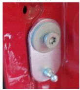
Tighten the bolt with the T50.
