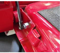
Periodically check the upper and lower mounting locations to insure that parts have not loosened through repeated use. If either mounting location is found to be loose, re-tighten the hardware as needed.
