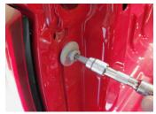
Install the bolt back through the hole in the ball mount into the vehicle.
