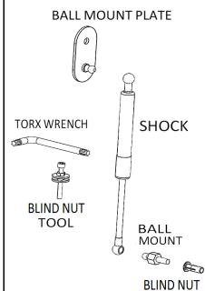
PARTS LIST: **ITEM** QTY THREAD LOCK TUBE SHOCK **BALL MOUNT PLATE BLIND NUT TOOL BALL MOUNT** BLIND NUT/NUTSERT TORX WRENCH MYLAR TOOLS REQUIRED: T-50 TORX M6 ALLEN WRENCH **16MM WRENCH** 13MM WRENCH TAPE MEASURE 16MM DEEPWELL SOCKET SUPERDUTY ONLY 8MM WRENCH
