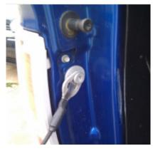
Install the bolt through the hole in the ball mount into the vehicle.
