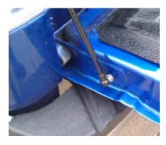
Periodically check the upper and lower mounting locations to insure that parts have not loosened through repeated use. If either mounting location is found to be loose, re-tighten the hardware as needed.
