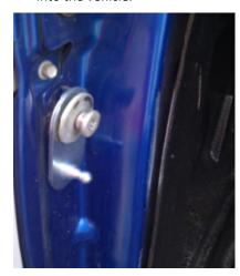
Tighten the bolt with the T50.
