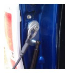
Install the narrow end of the shock on the ball mount.
