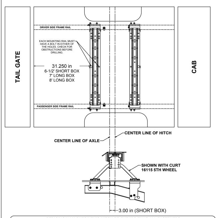
PERIODICALLY CHECK THIS HITCH TO ENSURE THAT ALL FASTENERS ARE TIGHT AND THAT ALL STRUCTURAL COMPONENTS ARE SOUND.
