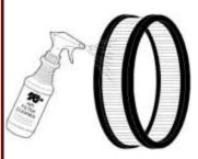
Spray K&N air filter cleaner liberally onto the entire element and let soak for 10 minutes.
