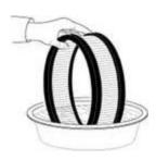
Large K&N elements can be rolled or soaked in a shallow pan of K&N air filter cleaner. Remove immediately and let sit for approximately 10 minutes.
