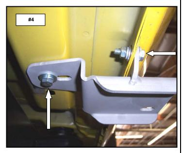
**STEP 4.** LOCATE THE HOLES IN THE BODY PINCH MOLD AND REMOVE THE TAPE COVERING THE THREADED HOLE IN THE UNDER SIDE OF THE BODY AT THE REAR OF THE VEHICLE. **PHOTO #5**
