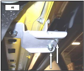
**STEP 8.** ALIGN THE SIDE STEP WITH THE VEHICLE AND TIGHTEN ALL MOUNTING BRACKET AND SIDE STEP NUTS AND BOLTS.
