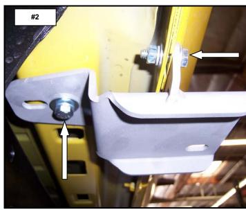
STEP 3. REPEAT THE ABOVE PROCEDURE TO INSTALL (1) 45052 MOUNTING BRACKETS AT THE CENTER POSITION. DO NOT TIGHTEN. PHOTO #3 & PHOTO #4
